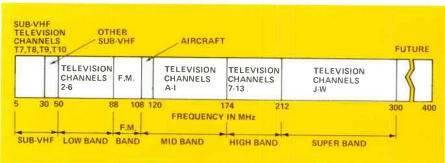
Figure 6. CATV Frequency Spectrum.
