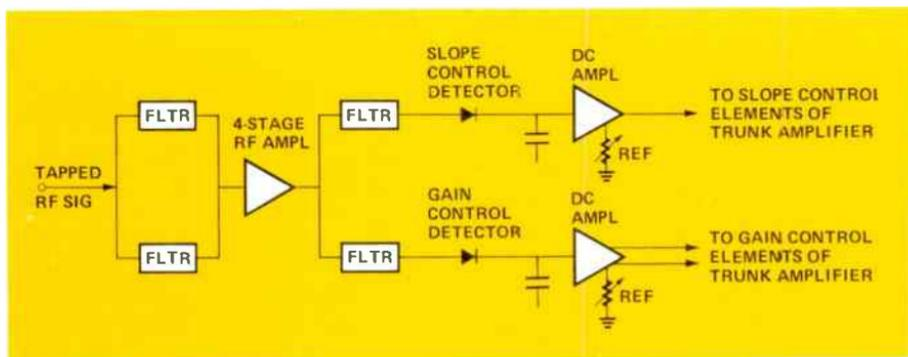
Figure 8. Automatic level and slope control circuit for total automatic control amplifier.
