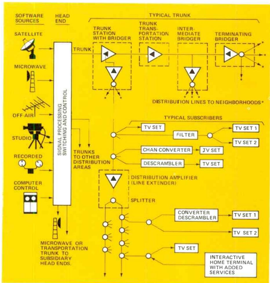
Figure 1. CATV system block diagram.
