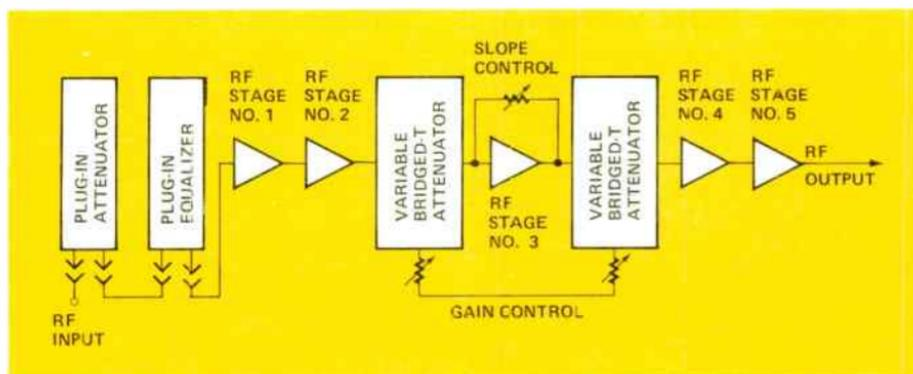
Figure 7. Basic trunk amplifier module.
