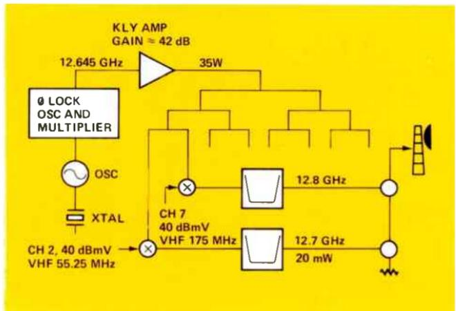
connected to the input of a multiplier chain to produce a final output,  $f_0$ , in the 12 GHz band (12.645 GHz in the figure). This signal is connected to one input of a mixer.
