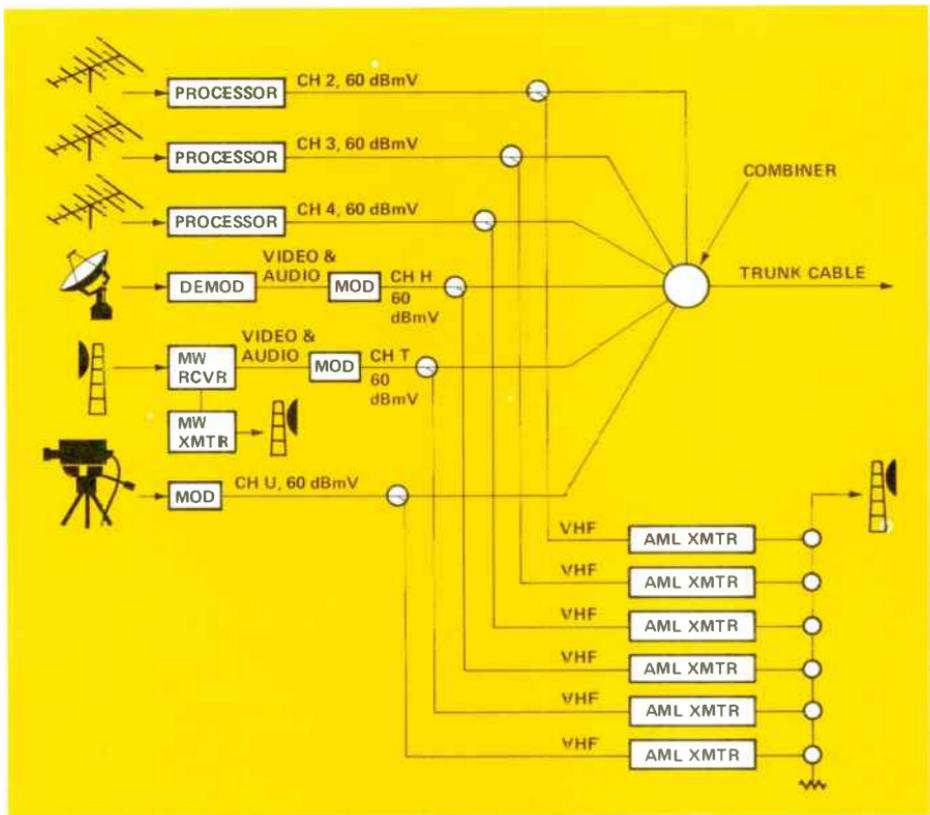
Figure 3. Block diagram for a head-end station.
