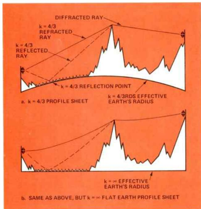
Figure 4. Ray tracings, flat and curved earth profile sheets.
