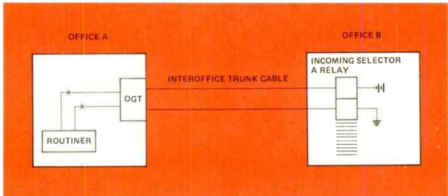
*Figure 1. Outgoing Trunk Number Completing Test*
