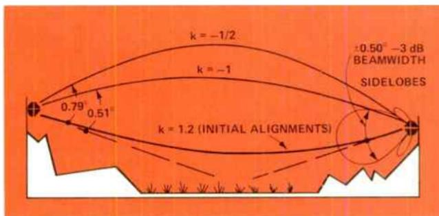
*Figure 5. Antenna decoupling on a 38-mile 6.7 GHz path traversing a swamp.*
