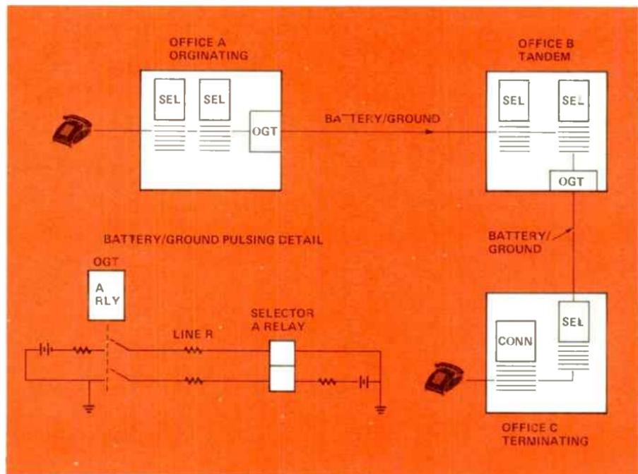
Figure 3. Tandem Physical Trunks
