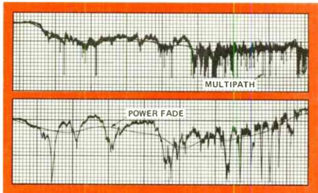
*Figure 1. Two examples of multipath fades superimposed on power fades.*
