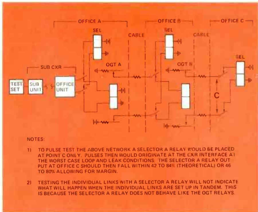
Figure 6. End to End Pulsing Test
