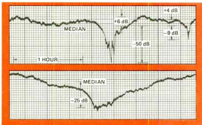
*Figure 2. Two examples of reflection only interference.*
