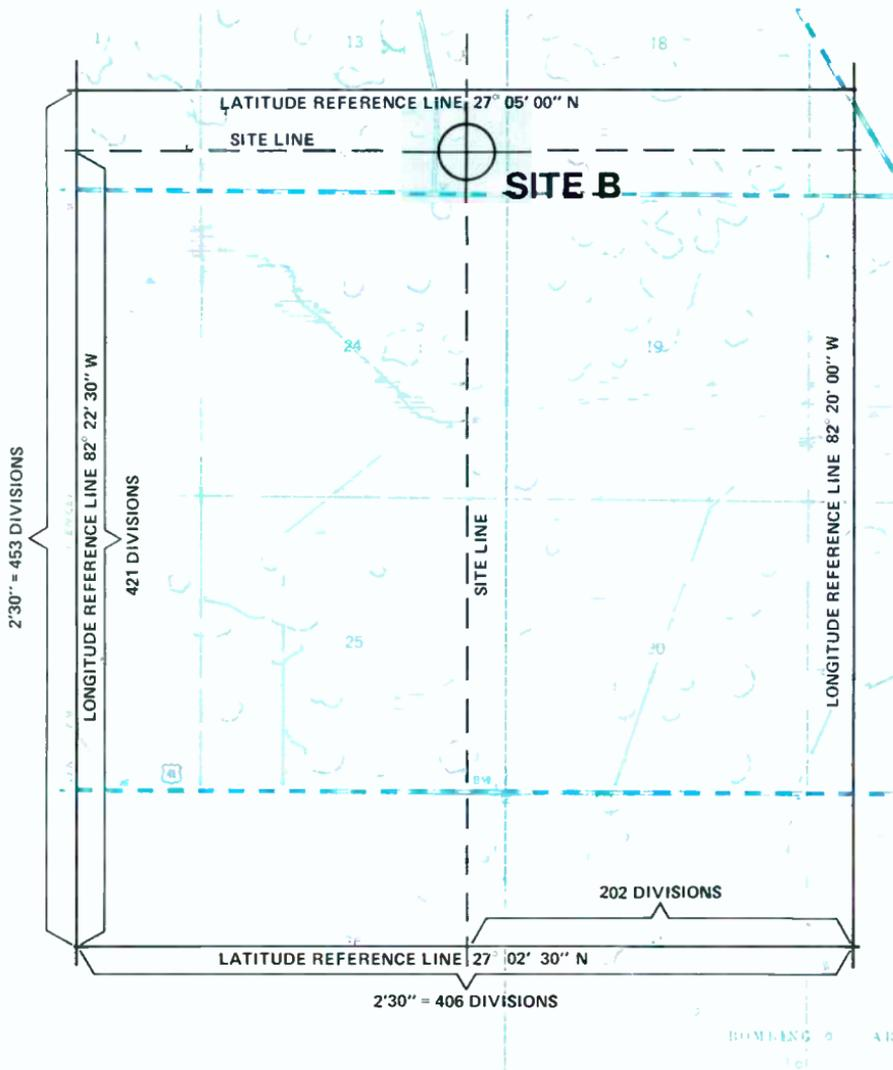
Figure 4. In the application of the ratio method the geographical coordinates of Site B are obtained from the solution of a proportion set up between two measurement ratios.
