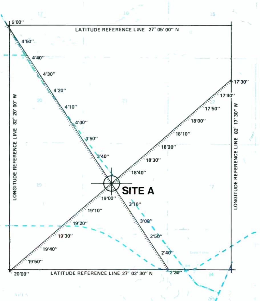
Figure 3. In the application of the direct reading method the geographical coordinates of Site A are read directly from the scale on the engineer's ruler.
