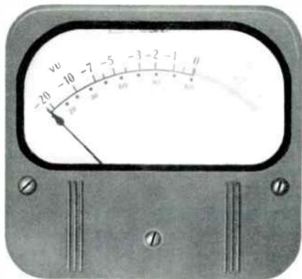
*Figure 1. The meter scale on the standard volume indicator is either the type A scale shown here, or the type B scale on which the positions of the vu and percentage scales are reversed.*
