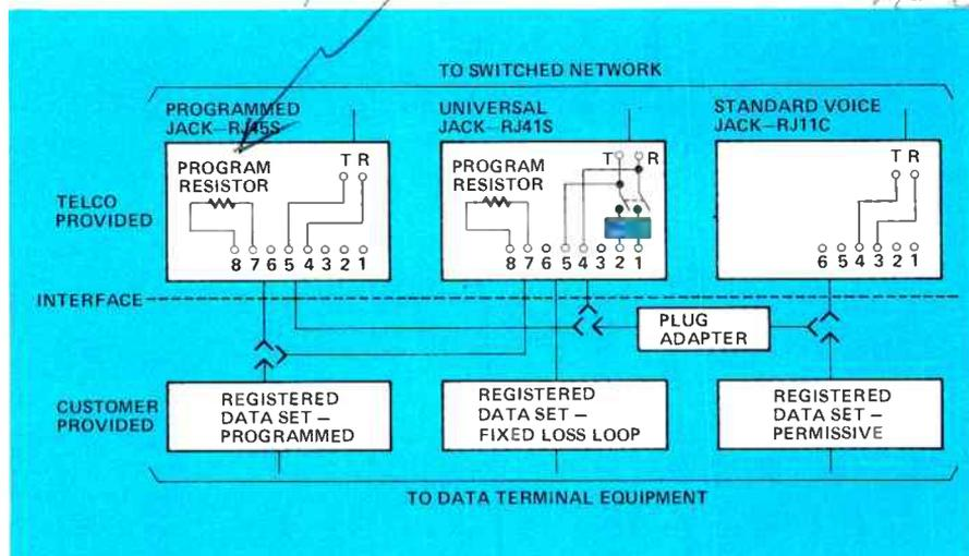
Figure 3. Part 68 of the FCC Rules and Regulations defines three classes of registered data sets based on output signal power of the data set.
