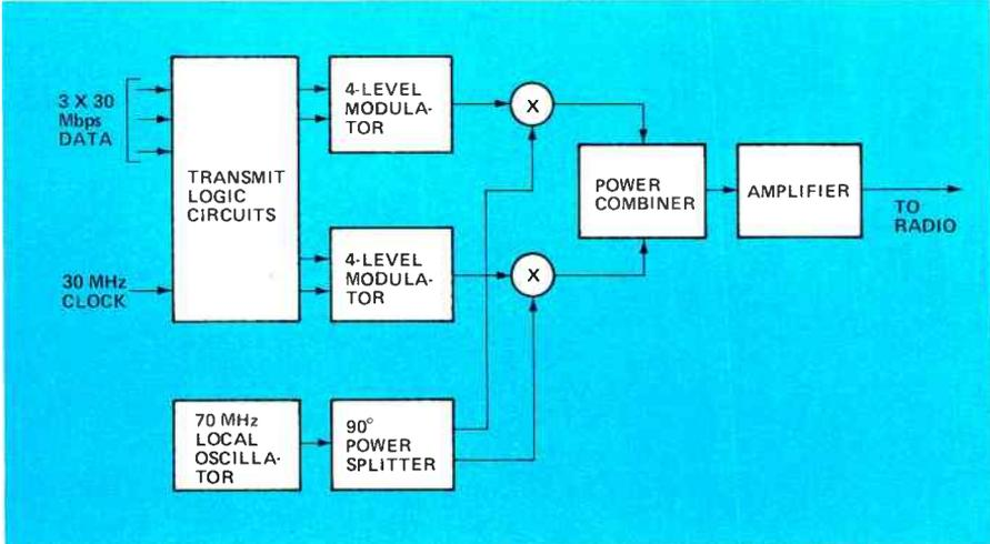
Figure 5. Block diagram of a modem transmitter in which 8 PSK modulation is used to modulate a 70 MHz intermediate frequency carrier.
