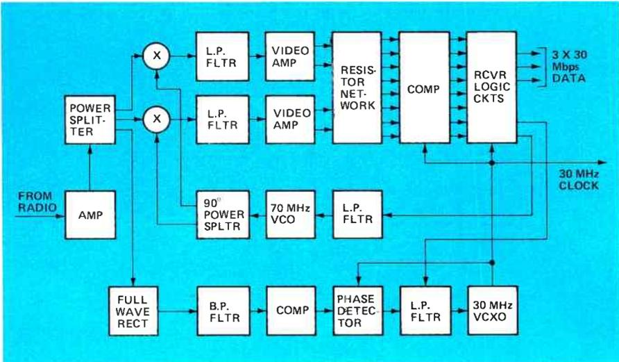
Figure 6. Block diagram of a modem receiver in which a 90 Mbps signal is recovered from a 70 MHz intermediate frequency carrier.
