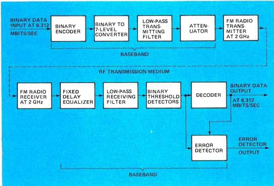
Figure 3. Block diagram of a 7-level modified duobinary digital transmission system over a 2 MHz FM radio.
