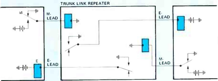
Figure 6. A typical trunk link repeater interconnecting two trunks which have incompatible E&M signaling interfaces.
