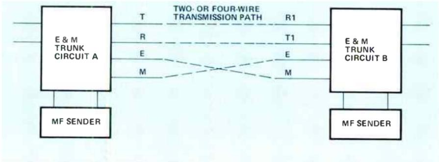
Figure 3. Block diagram of a multifrequency signaling system with E&M leads.
