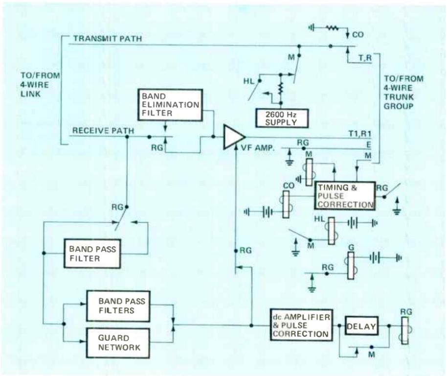
Figure 2. A typical SF signaling system using 2600 Hz as the signaling frequency. The primary function of the vf amplifier is to prevent noise or speech from interfering with the operation of the signal detector.
