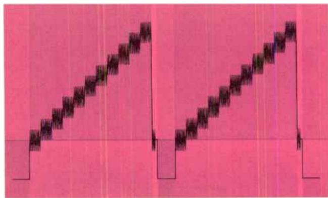
*Figure 6. Typical staircase test signal, with simulated color subcarrier impressed, which can be used to detect nonlinearities, and to measure differential phase and gain, in a video system.*
