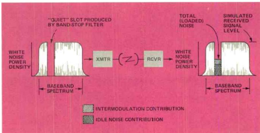
*Figure 1. The loaded noise measured in a test slot is the product of both intermodulation and idle noise contributors. Depending upon the location of the slot in the spectrum and the characteristics of the contributors, the source of an impairment can be identified.*
