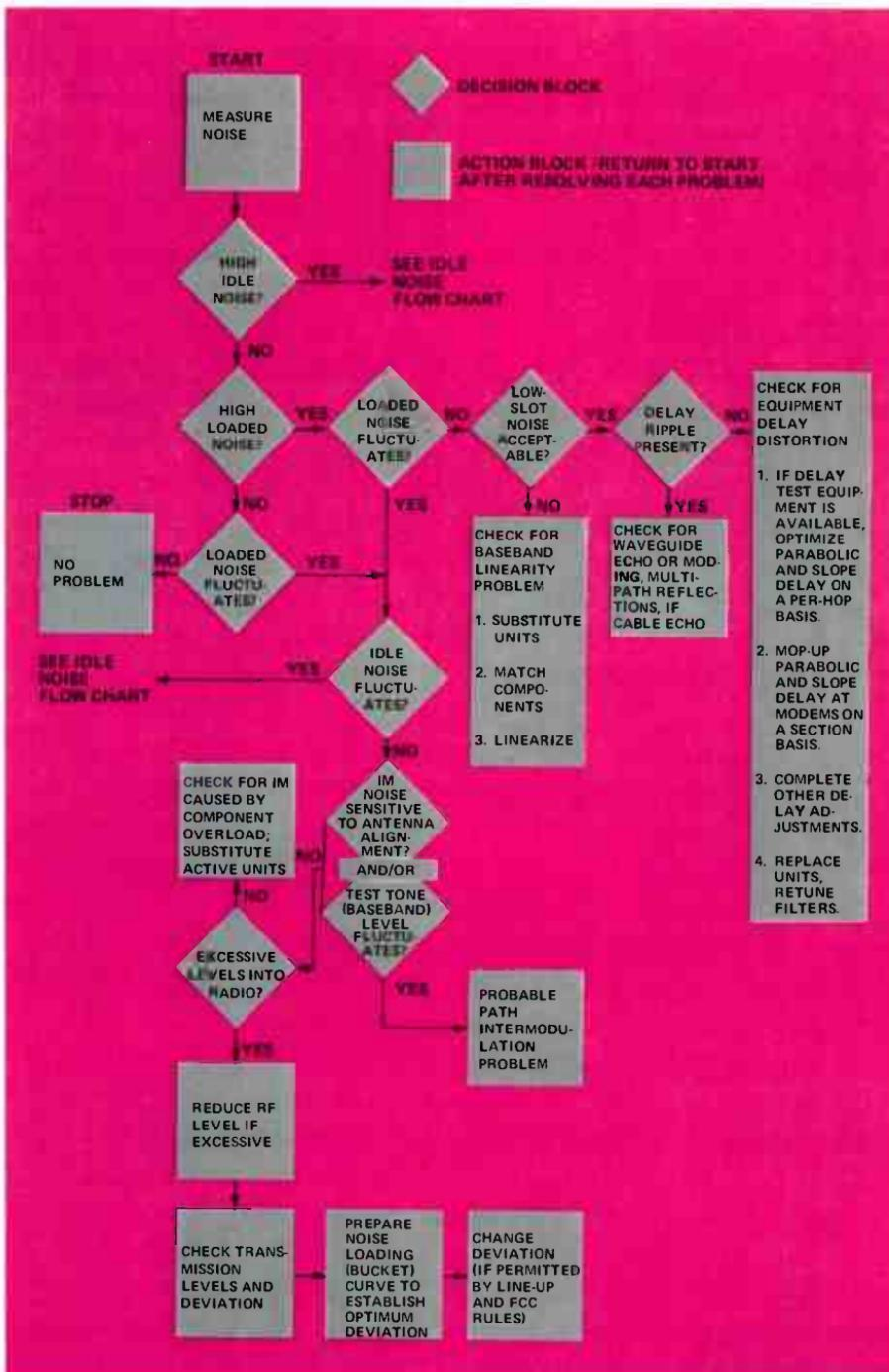
Figure 3. A loaded noise flow chart is a logical progression of steps taken to isolate the cause of a high loaded noise measurement.
