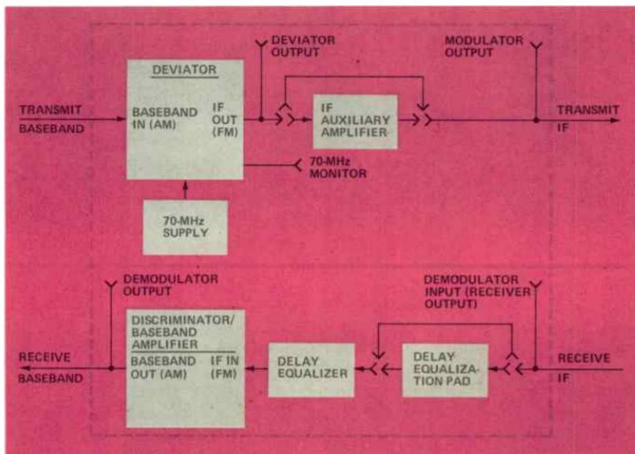
Figure 2. An IF modem interface is included in heterodyne systems. In remodulating systems, deviation and discrimination are performed within the transmitter/receiver equipment.
