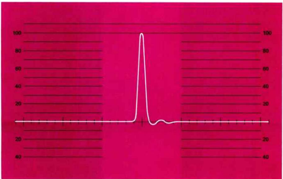
*Figure 8. Ringing due to bandwidth constriction will appear as a series of peaks following the  $\sin^2 (2T)$  pulse.*
