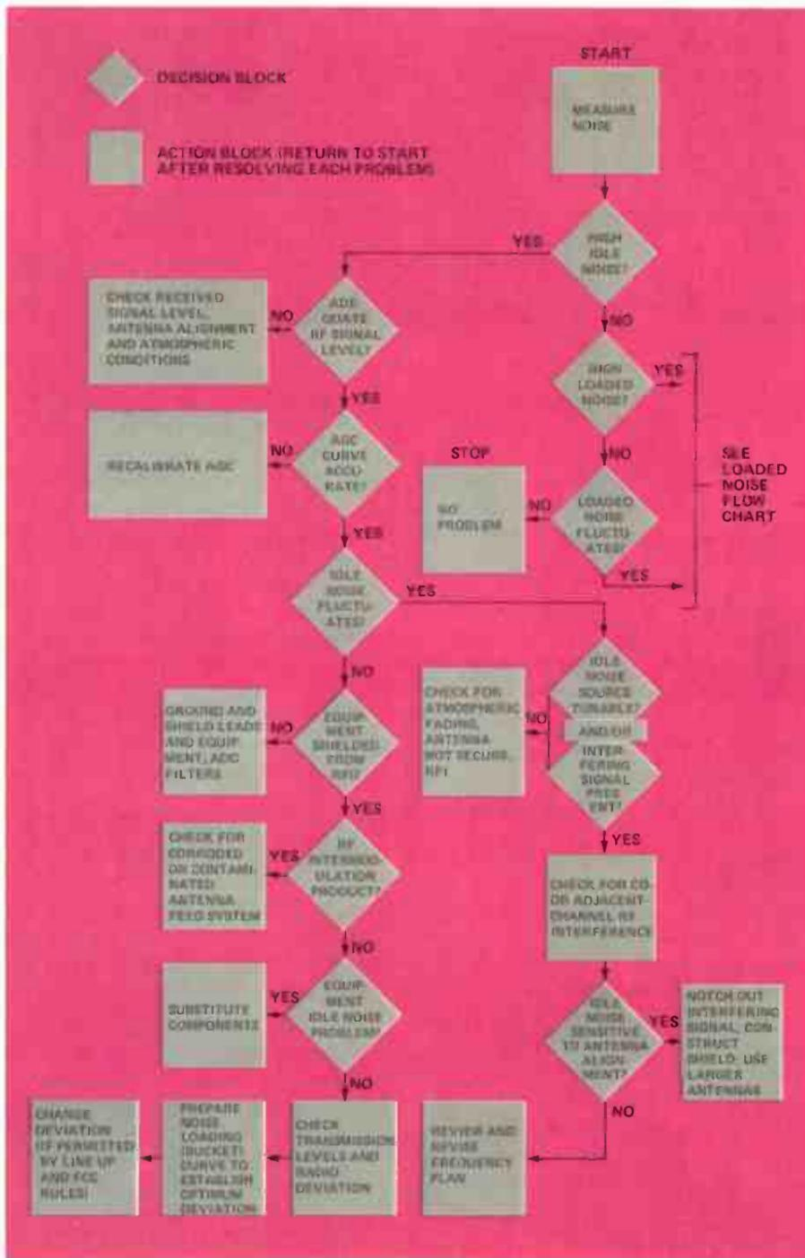
*Figure 2. An idle noise flow chart can be of considerable value when attempting to isolate the source of a high idle noise measurement.*
