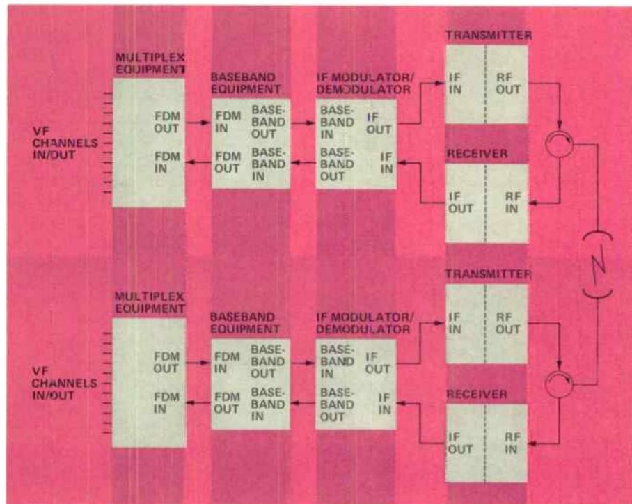
*Figure 1. In a microwave radio system such as the simple heterodyne type shown, there are many points at which signal degradation can occur.*
