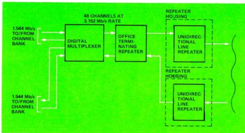
*Figure 3. A typical 48-channel PCM cable carrier system requires a digital multiplexer to combine two 24-channel signals. It also requires new repeaters and repeater housings, and is thus generally used only in new installations.*
