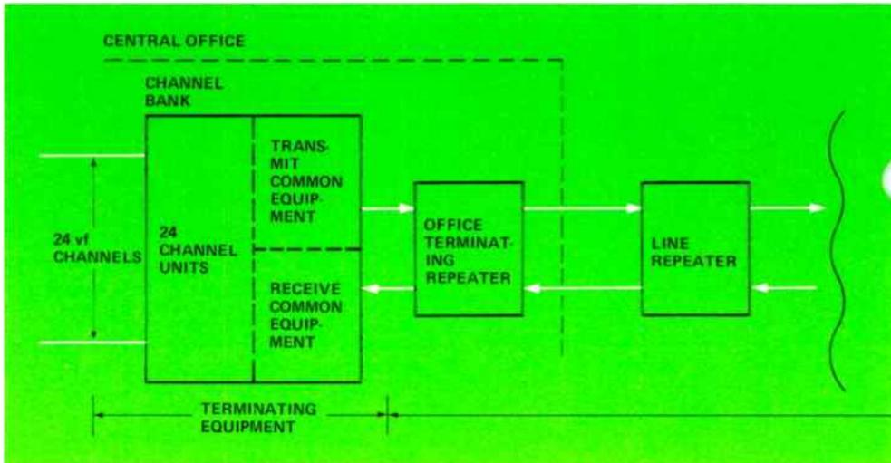
Figure 1. A typical 24-channel, T1-type PCM cable carrier system is composed of terminating equipment, in the form of channel banks, in two central offices linked by a span, or repeatered, line.
