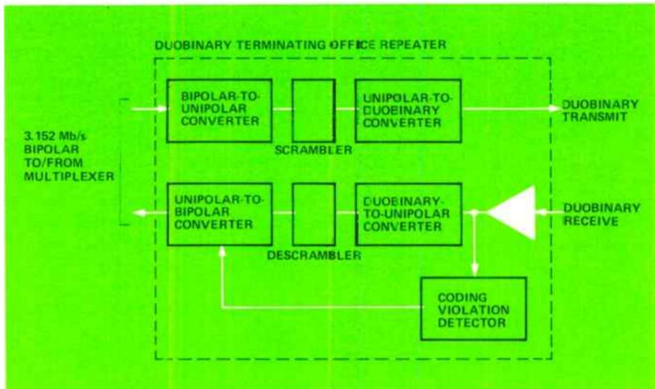
Figure 6. The duobinary end, or terminating, office repeater contains the bipolar-to-duobinary conversion interface that makes possible 48-channel transmission on facilities originally designed for only 24 channels.
