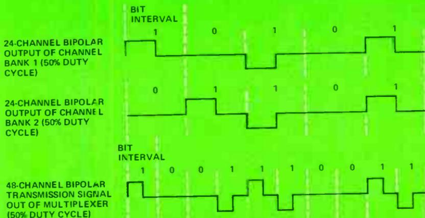
A. BIPOLAR CODING TO ACHIEVE 48-CHANNEL PCM SYSTEM CAPACITY.
