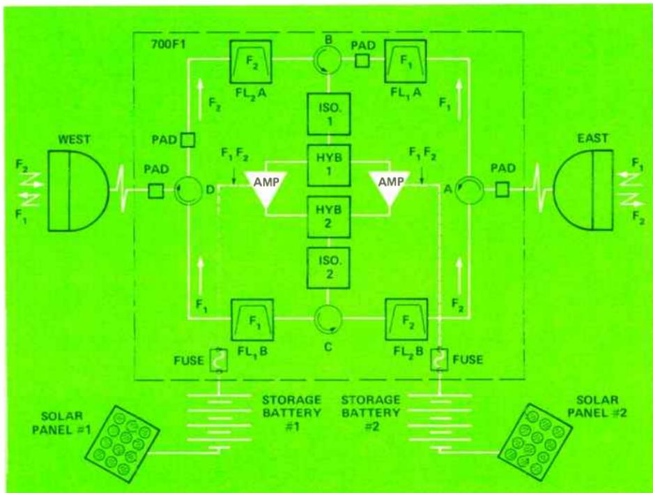
Figure 1. Component diagram of the GTE Lenkurt rf repeater.
