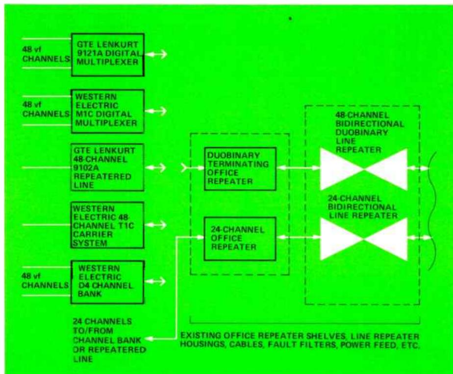
Figure 5. The duobinary repeatered line can accept its 3.152-Mb/s input from many sources, and can operate in the same cable as 24-channel systems.
