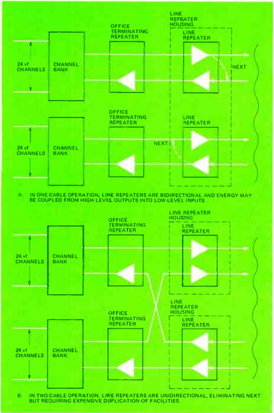
Figure 2. Line repeaters can be made bidirectional or unidirectional by proper orientation of their regenerator sections.
