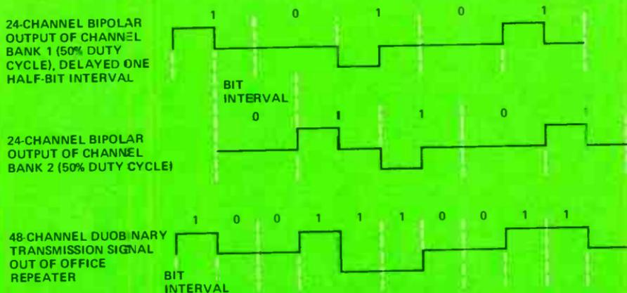
B. DUOBINARY CODING TO ACHIEVE 48-CHANNEL PCM SYSTEM CAPACITY CAN BE CONCEPTUALLY VISUALIZED AS TWO INTERLEAVED T1-TYPE PULSE STREAMS.
