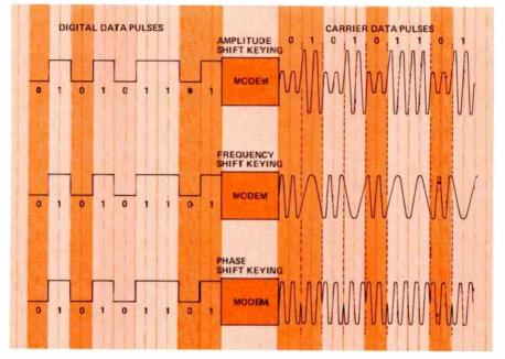
Figure 2. Three basic modulation techniques are available for translating digital data into a form more compatible with telephone system transmission facilities.
