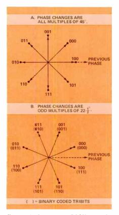
Figure 4. In 8-phase DPSK modulation, a data pulse can assume one of eight phase angles with respect to the phase of the preceding pulse. Each phase represents a different group of three binary digits (tribits).
