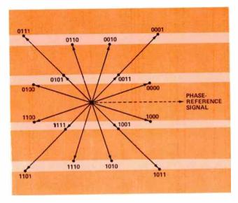
Figure 6. Quadrature amplitude modulation combines phase and amplitude shifts to produce a complex set of signal state choices, each of which represents a different 4-digit binary number.
