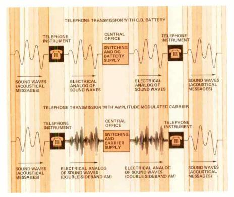
Figure 1. A voice-channel telephone facility converts acoustical messages into an electrical analog suitable for transmission on the telecommunications network.
