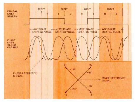
Figure 3. In multiphase PSK, each shift represents more than one information bit.
