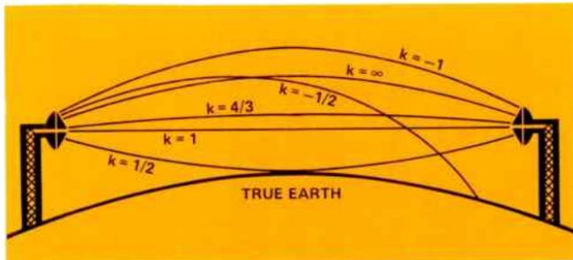
than one, the beam curves upwards or opposite to the curvature of the earth; to the microwave beam, the earth appears to “bulge.” The effect of earth’s bulge may be to partially obstruct the transmission path, causing an obstruction or diffraction. The curvature for various values of  $k$  can be calculated from the relationship:
