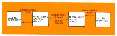
Figure 1. The subscriber's loop connects the telephone to the central office.
