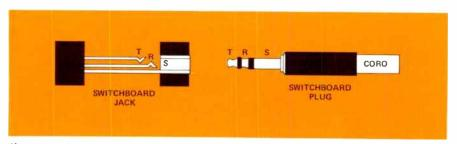
Figure 3. The tip (T), ring (R), and sleeve (S) designations of a telephone line originated from the contact descriptions on a telephone plug.
