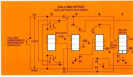
Figure 4. Trunk circuit using reverse-battery signaling.
