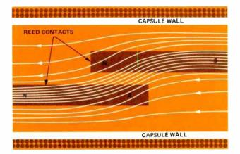
Figure 9. Magnetic lines of force in a correed relay.
