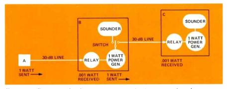
Figure 4. The use of relays in a communication network reduces power requirements as well as the possibility of human error.
