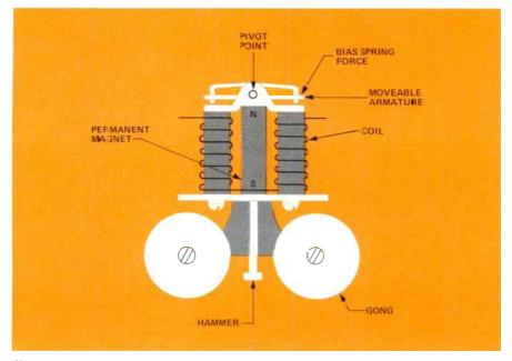
Figure 10. Typical telephone ringer arrangement.
