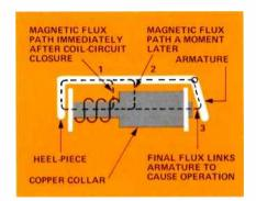
Figure 5. Magnetic flux paths in an armature-end collar relay.
