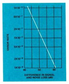
Figure 5. The error rate of an office repeater is governed by the difference between noise path loss and signal path loss in the end-section of a repeatered line.
