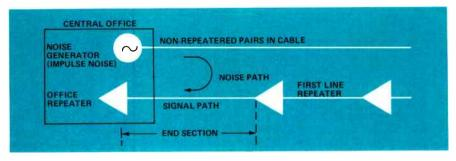
Figure 4. More conservative end-section repeater spacing is required with an increase in tandem spans.
