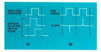
Figure 1A. Phase jitter causes a variation in the phase of the PCM signal.
