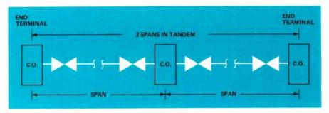
Figure 2. As it becomes necessary to increase the length of repeatered lines, several spans can be placed in tandem.
