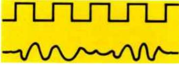
**Is it digital, digitized-analog, or analog? These distinctions need to be understood when designing and using telecommunications equipment.**
