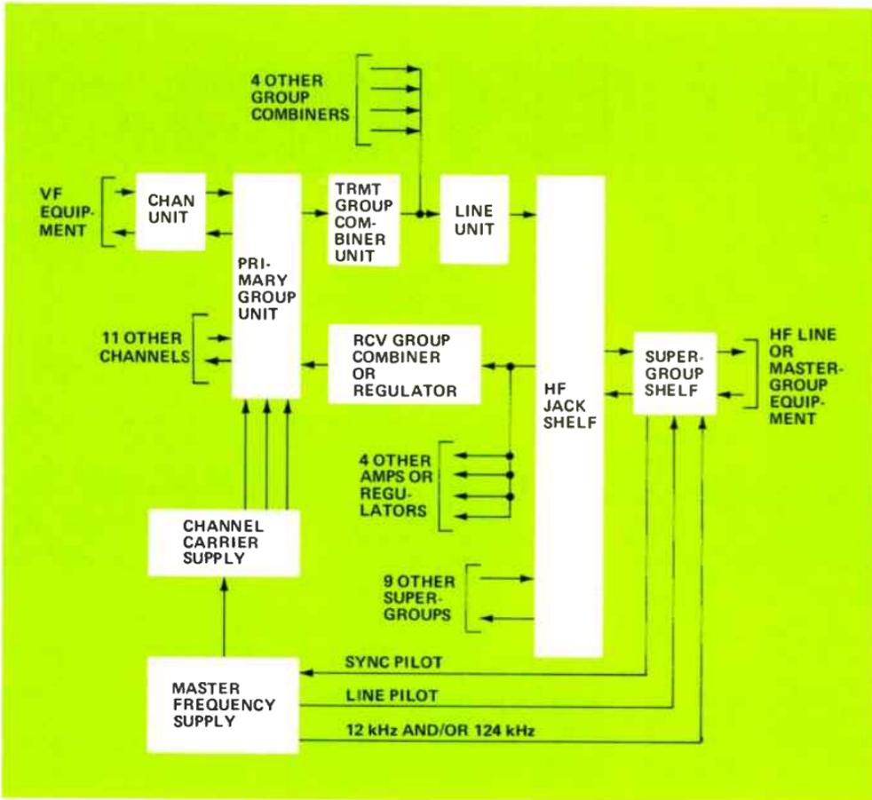
Figure 7. Typical DFSG terminal configuration.
