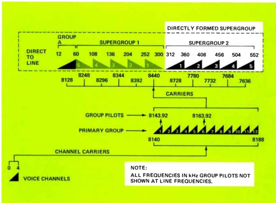
Figure 5. Direct-to-line and directly-formed supergroup modulation plans.
