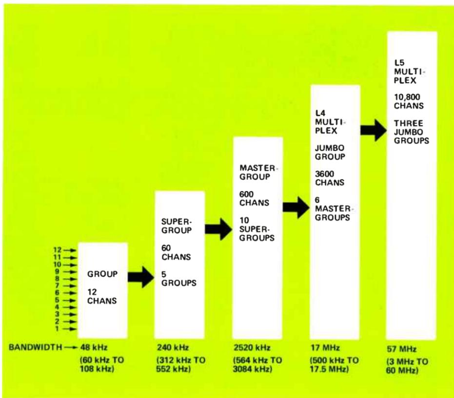
Figure 2. The hierarchy of FDM terminals.
