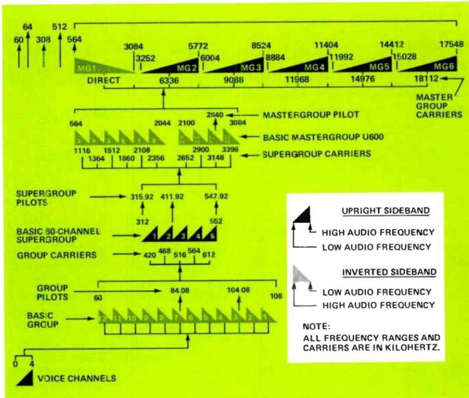
Figure 3. Conventional FDM frequency allocation and modulation.
