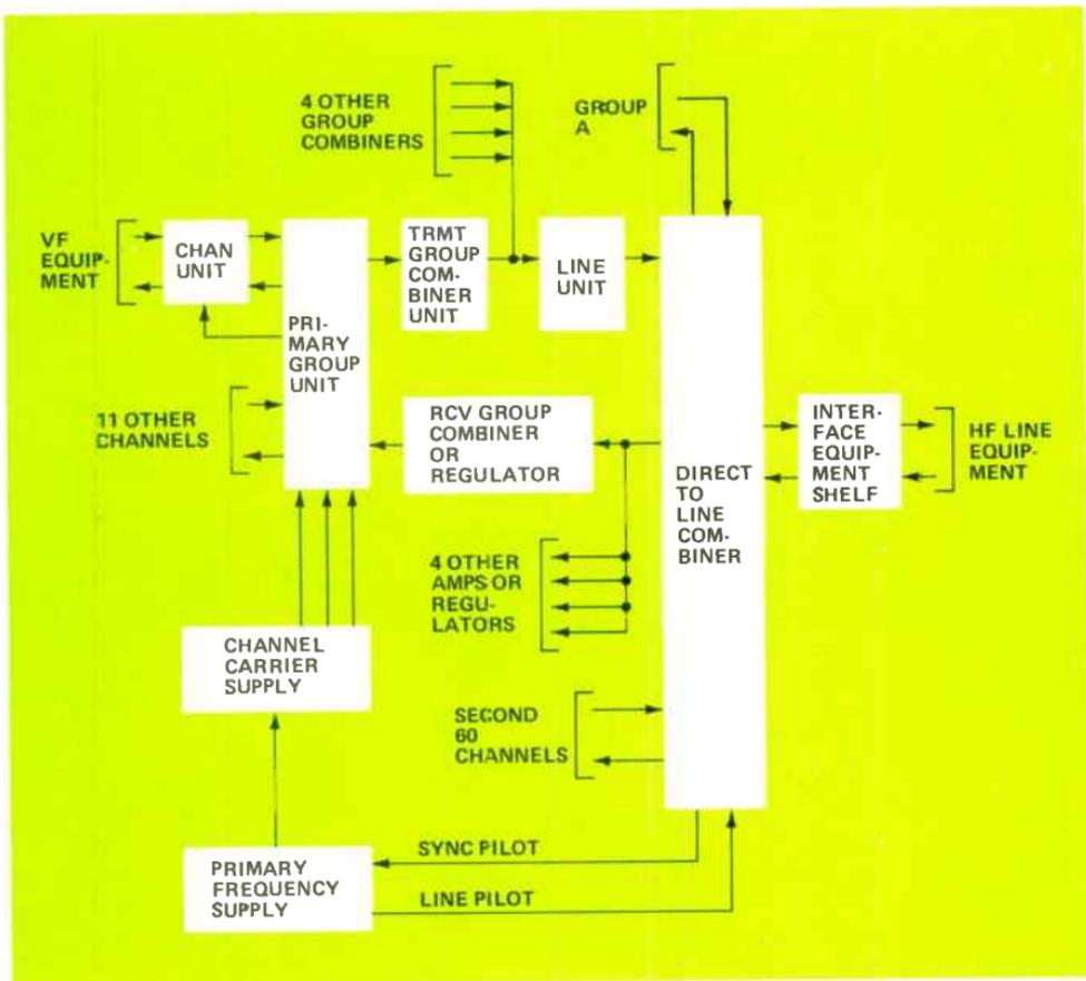
Figure 6. Typical DTL terminal configuration.
