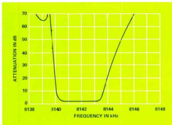
Figure 4. Typical passband of a poly-lithic crystal filter.
