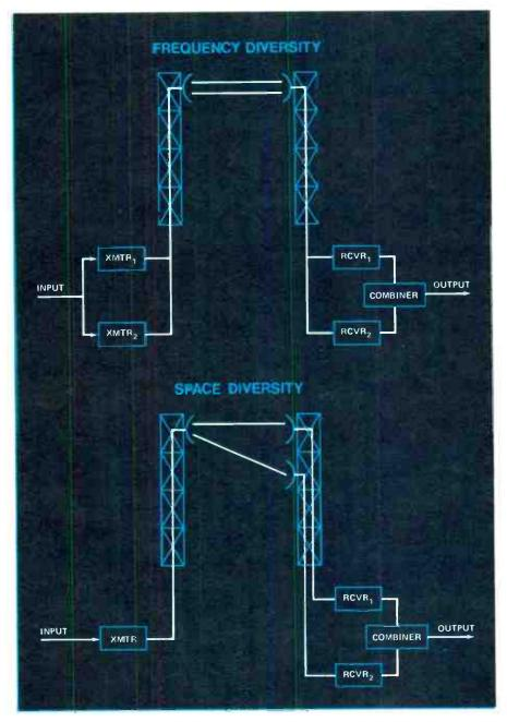
Figure 1. Frequency diversity and space diversity accomplish similar ends but they use different equipment configurations.
