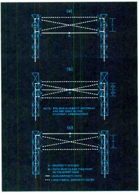
Figure 2. In the most conservative space diversity arrangement (a) with all the spacing above the existing antenna, all paths give adequate clearance: when the spacing is split above and below the existing antenna (b), three out of four paths are good: and when all the spacing is below (c), only the top-to-top path is good.
