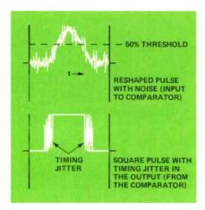
Figure 4. The voltage comparator circuit detects the presence or absence of pulses.
