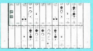
The 758B baseband equipment provides various forms of operating characteristics to condition broadband multiplex and video signals for transmission over microwave systems such as the GTE Lenkurt type 75 and the type 78 radio families. For more information, write GTE Lenkurt, Dept. C134.
