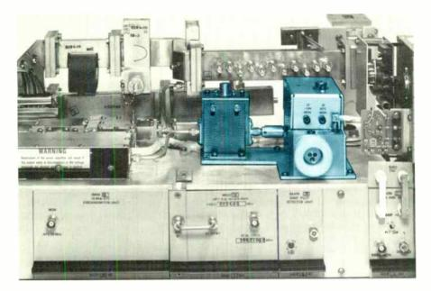
Figure 1. The replacement of the klystron with a solid state microwave source is one of the major changes in GTE Lenkurt microwave radios.
