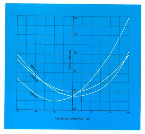
Figure 6. Typical overall noise performance for a GTE Lenkurt type 78A2, 1200-channel baseband radio, in a 6-hop system.
