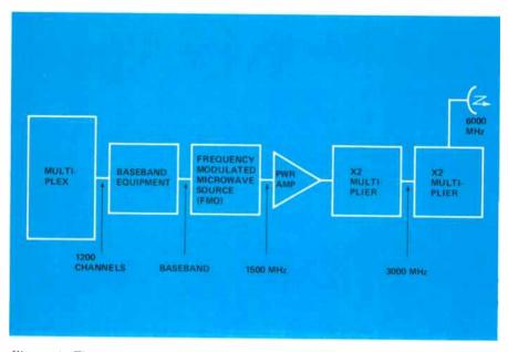
Figure 4. The transmit section of a baseband microwave radio terminal working with telephone multiplex equipment.
