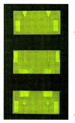
Figure 4. After etching, microstrip substrates are ready for the mounting of discrete components.
