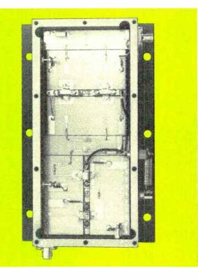
Figure 5. Hybrid microstrip circuits in a microwave power amplifier.
