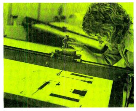
Figure 3. The first step in the construction of a microstrip circuit is the drawing of the dimensional pattern at ten times its normal size.
