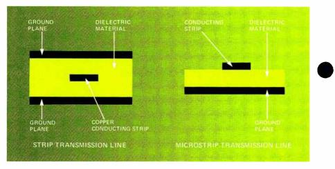
Figure 2. Microstrip transmission lines differ from strip transmission lines in construction as well as in size and type of material.
