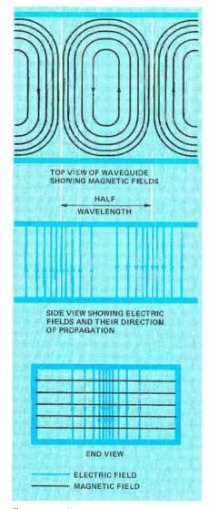
Figure 3. Field configuration of the dominant mode in rectangular waveguide.
