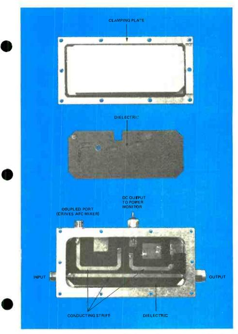
Figure 8. The principal of the strip line is used in construction of directional couplers.
