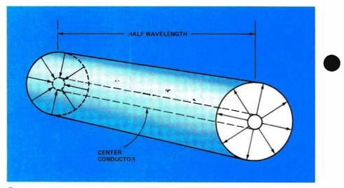
Figure 2. In coaxial transmission line, the electric fields are in opposite directions at each half-wavelength.
