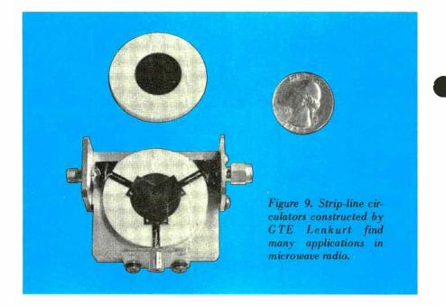
ly used at lower radio frequencies become extremely small and inefficient at microwave frequencies. Microwave circuitry is therefore often manifested in lengths of transmission line rather than discrete components. By designing strip lines of various lengths and patterns, it is possible to achieve results which are equivalent to those obtained by conventional components at lower frequencies.
