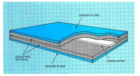
Figure 4. General configuration of a strip transmission line.
