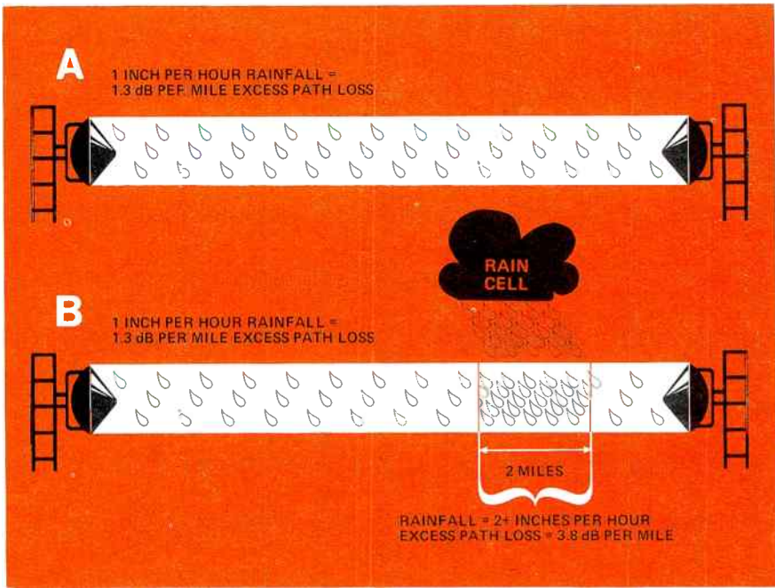
Figure 6. Raising the fade margin by 5 dB, (as in B above) can permit transmission through a rain cell of substantially greater intensity.
