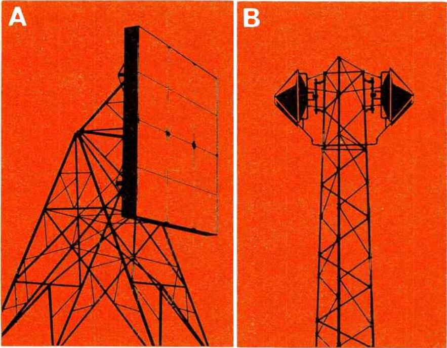
*Figure 2. Passive repeaters are of two basic types: the “billboard” (A), so labelled because of its appearance, and the parabolic “back-to-back” passive (B) which uses two standard antenna dishes directly joined by a short length of waveguide.*
