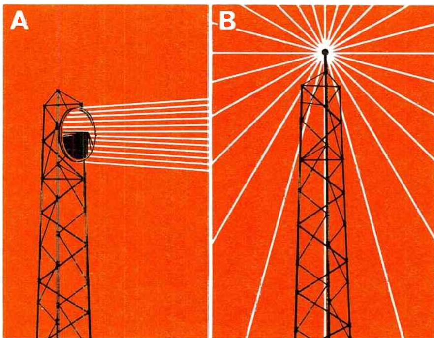
*Figure 3. Energy radiation is theoretically assumed to radiate isotropically in all directions (B). Parabolic antennas are used to focus radiant energy into a directional beam (A) which has an obviously high amplitude gain over the hypothetical isotropic antenna.*
