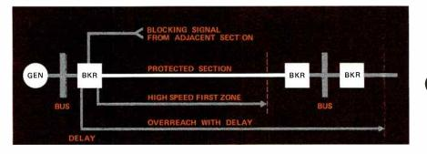
Figure 5. Typical "overreach" arrangement with third zone blocking. High speed distance relays at both ends detect first zone faults. Sensitivie overreach relay detects second zone faults, but is blocked by signal from far end which indicates when the fault comes from the adjacent section. A slight delay is built into the overreach circuit to allow the blocking signal to have "first priority" in acting.
