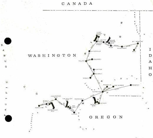
Figure 1. The Bonneville Power Administration's EHV network in the Pacific Northwest is typical of modern extensive power transmission systems. Recently, consideration is being given to creating an intertie between this network and a similar one in the Southwest.
