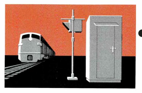
Figure 4. Mounted at trackside so as to provide maximum view of the passing trains, the scanner covers a vertical area of just under nine feet. Its protective housing allows the scanner to operate at temperatures ranging from  $-50^{\circ}$  to  $150^{\circ}$  Fahrenheit.
