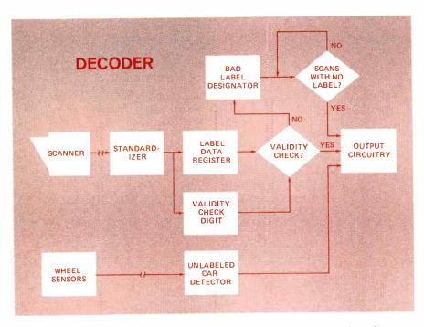
Figure 6. Primarily, the decoder's job is to receive the color signals and convert them into meaningful electrical impulses for transmission as data.
