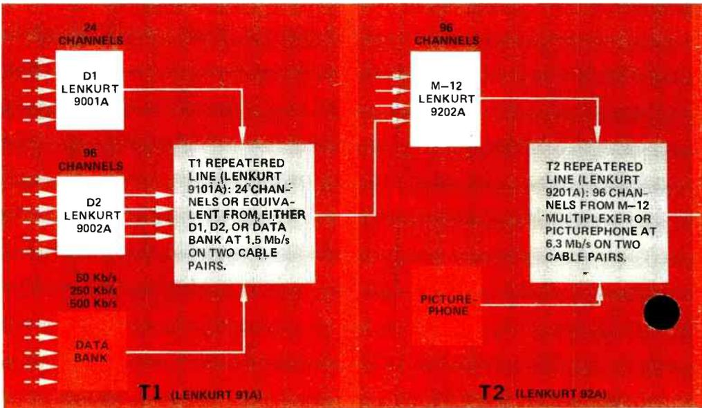
Figure 2. PCM systems, expanding from T1 to T4, will mix voice and other
