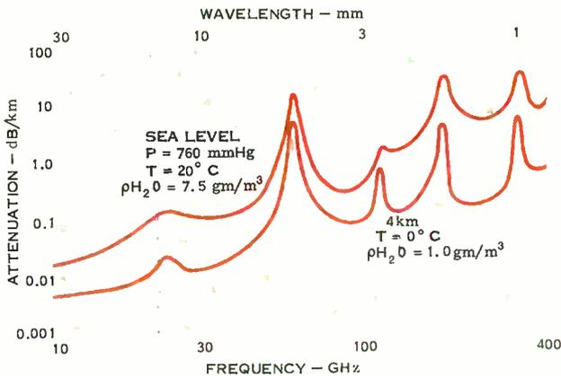
Figure 3. Attenuation of high frequencies at different altitudes is affected by oxygen and water vapor.  $P$  indicates barometric pressure,  $T$  atmospheric temperature and  $\rho H_2O$  is water vapor density.
