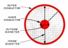
Figure 2. Coaxial tube dimensions are specified by the outside diameter of the inner conductor, and the inside diameter of the outer conductor.
