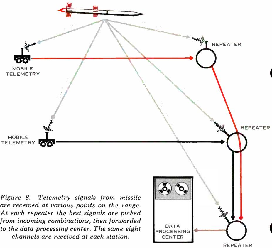
*Figure 8. Telemetry signals from missile are received at various points on the range. At each repeater the best signals are picked from incoming combinations, then forwarded to the data processing center. The same eight channels are received at each station.*
