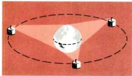
*Figure 1. Three satellites in synchronous orbit could cover the entire earth.*
