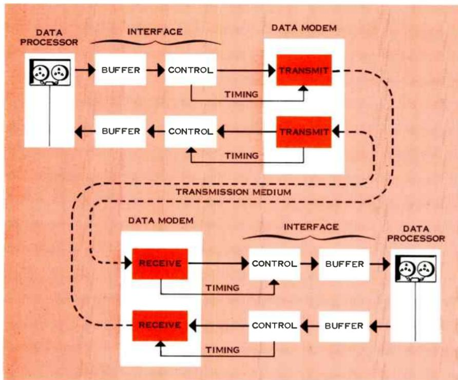
Figure 1. Typical full-duplex data transmission system arrangement. Timing signals from control unit synchronize data transmitter with data processor. At receiver, the element of time is important in reconstructing the original digital representation of the data. This is accomplished by deriving sync pulses from the data stream.
