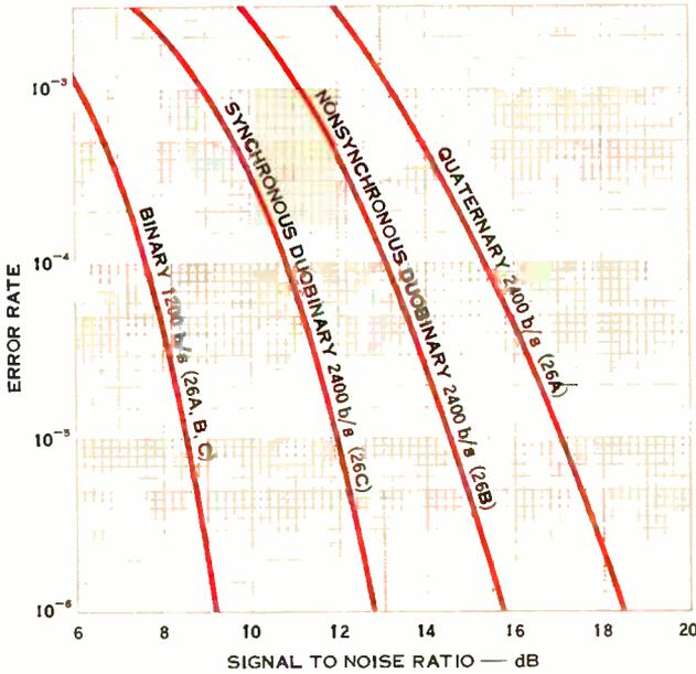
Figure 4. Comparison of error rate versus signal-to-noise ratio. Without normalization synchronous Duobinary has a noise penalty of about 3.4 dB compared to binary. This is a marked increase in performance over nonsynchronous Duobinary and quaternary.
