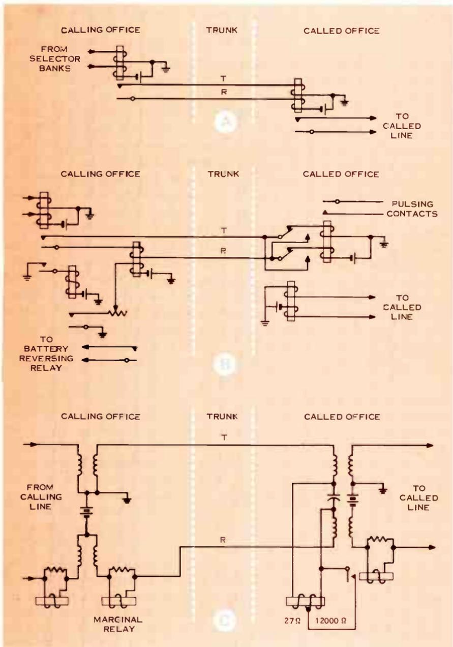
Figure 1. Loop signaling is accomplished by altering the flow of current in the trunk conductors. Three methods used to accomplish loop signaling are: (A) wet-dry, (B) reverse battery, and (C) high-low.
