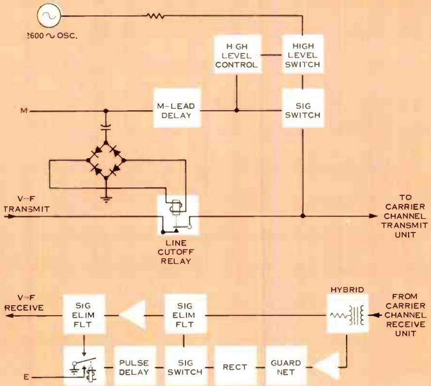
Figure 3. Simplified block diagram of a 2600-hz in-band signaling circuit applied to transmit channel and receive channel of a carrier system.
