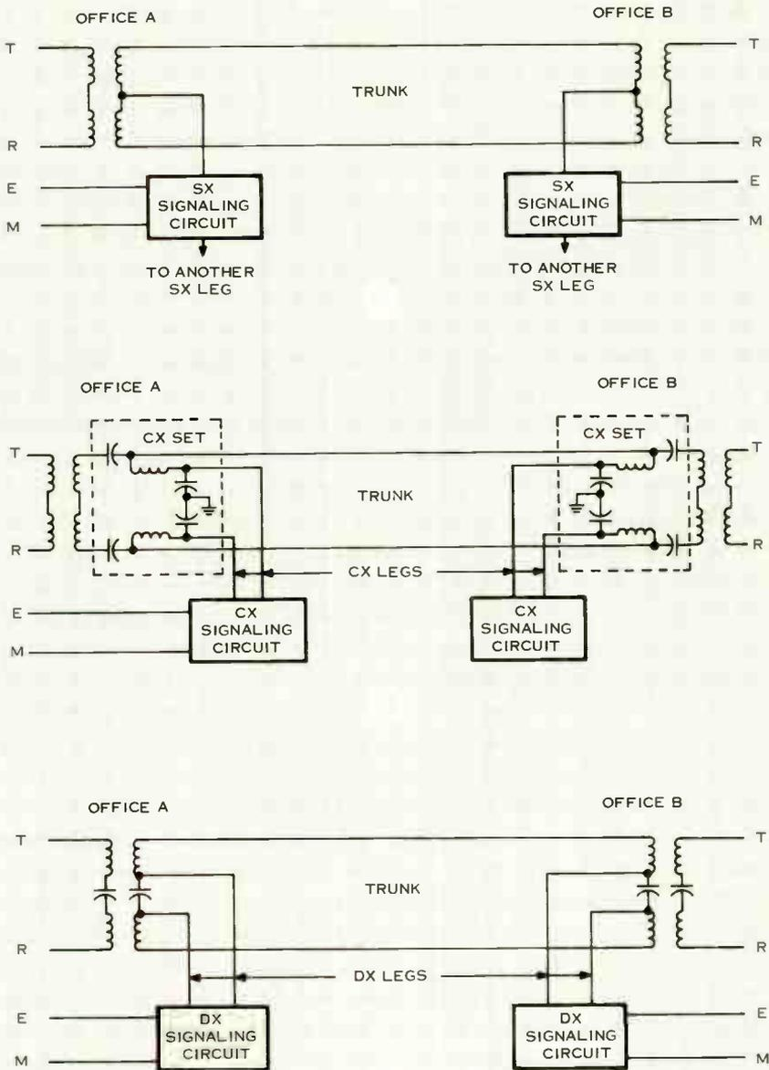
Figure 2. There are a number of different circuit arrangements designed for E & M signaling over telephone trunks. The three most prominent d-c arrangements are: (A) simplex, (B) composite, and (C) duplex.
