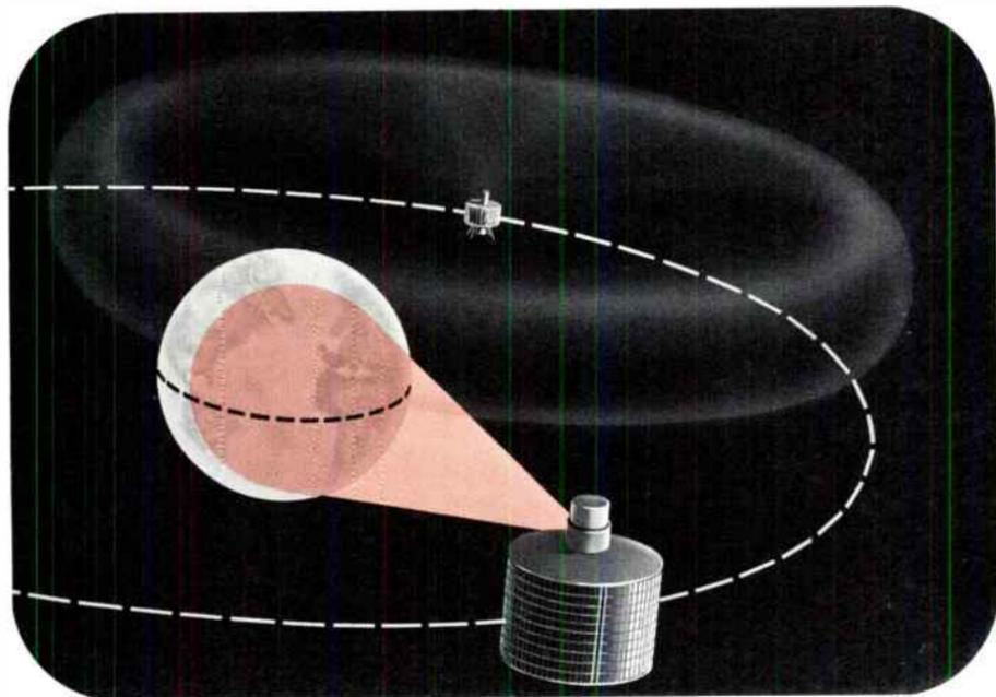
*Figure 2. Toroidal pattern of first communications satellites (rear) loses much rf energy to space. Intelsat 3 will focus its communications beam toward earth, using new despun antennas, with up to 16 dB gain.*
