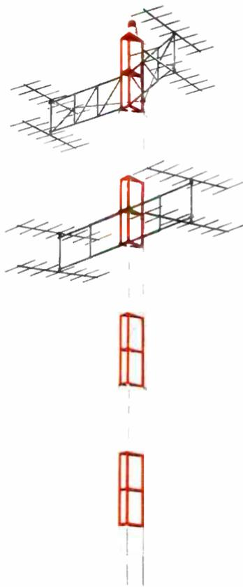
*Figure 1. High gain Yagi antennas, one for each television station, receive off-the-air signals to be relayed through CATV system.*
