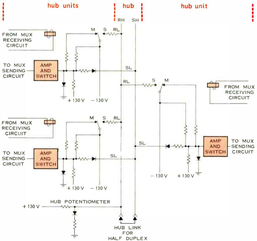
Figure 5. Hub operation, showing three multiplex telegraph channels interconnected on the d-c loop side.
