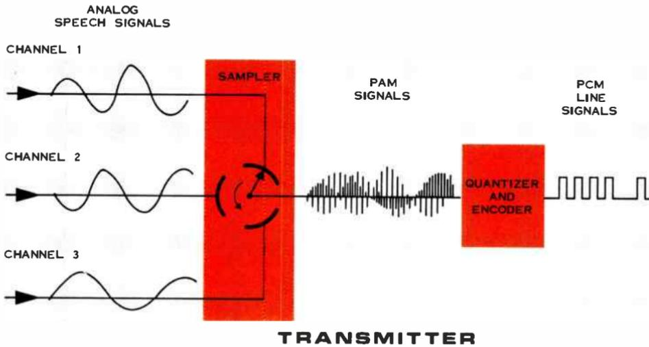
Figure 2. Simplified time division multiplex PCM system.
