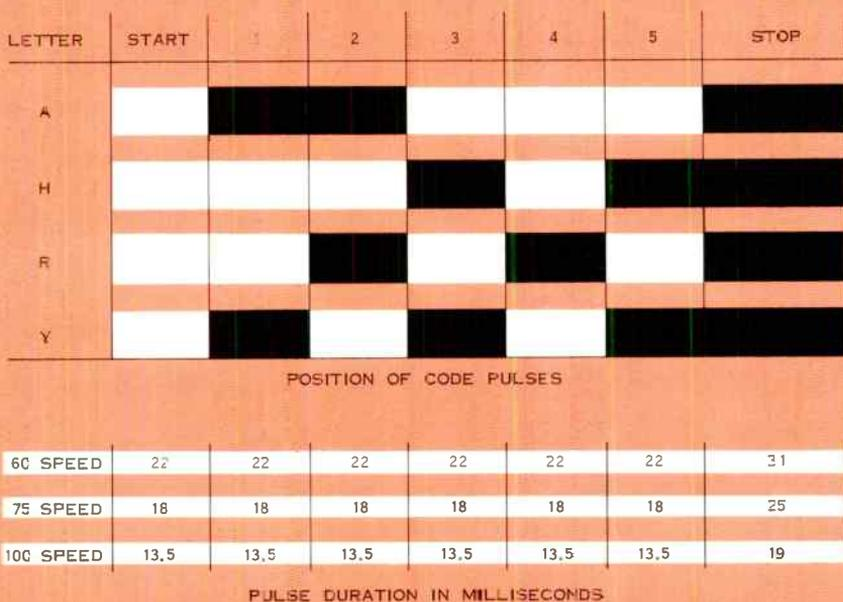
Figure 1. Examples of the 5-level Baudot code for the letters A, H, R, and Y, including pulse lengths for the three standard telegraph speeds. Mark pulses are shown in color while space pulses are shown in white.
