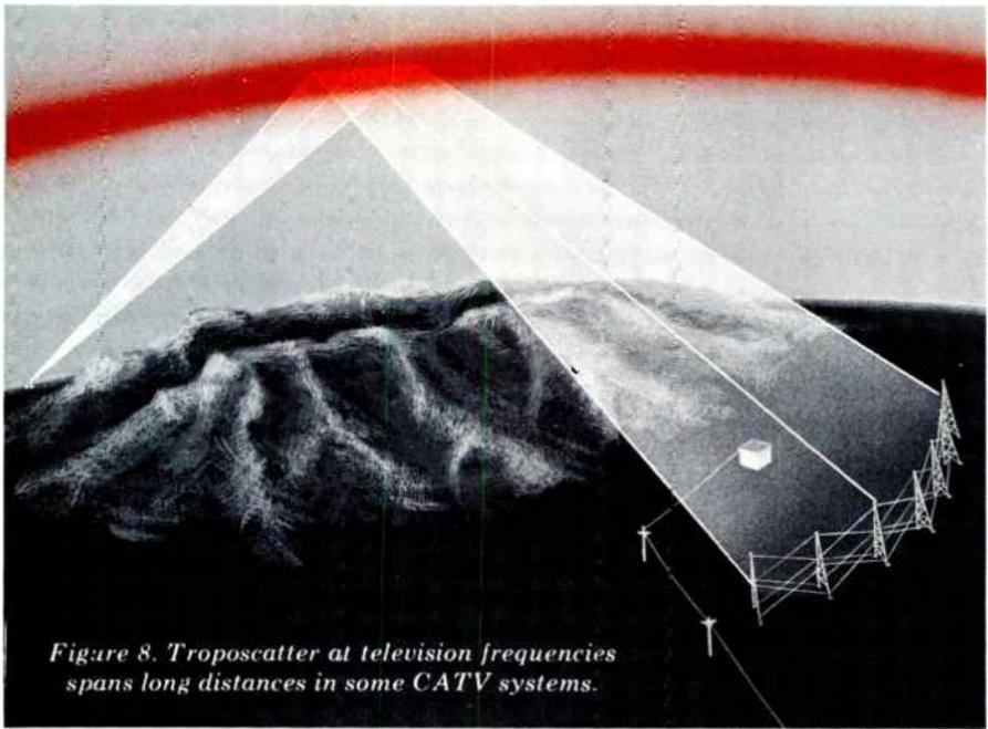
*Figure 8. Troposcatter at television frequencies spans long distances in some CATV systems.*
