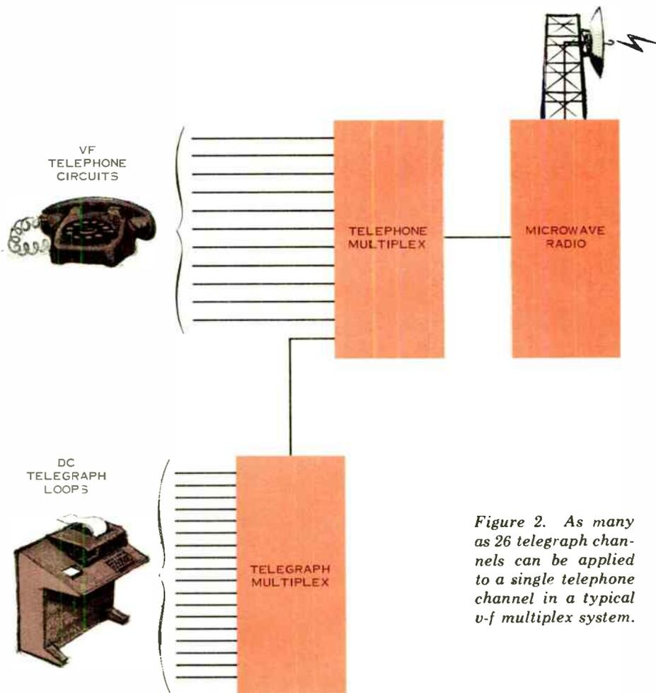
*Figure 2. As many as 26 telegraph channels can be applied to a single telephone channel in a typical v-f multiplex system.*
