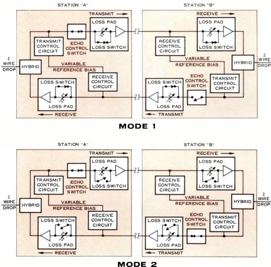
Figure 4. Simplified diagram of Mode 1 (uni-directional) and Mode 2 (bi-directional) operation of the Lenkurt 931B Echo Suppressor.
