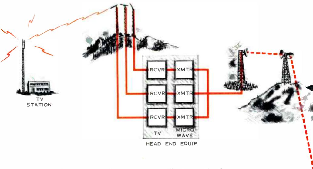
Figure 5. CATV system picks up signals outside the reach of home antennas; may use microwave radio to relay them to cable distribution point. Utility poles carry coaxial cables through residential areas.
