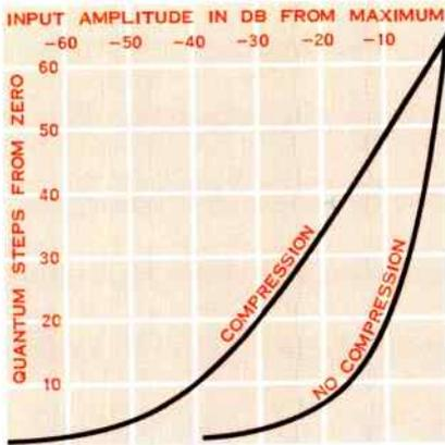
Figure 4. Signal compression using typical logarithmic compression characteristic.
