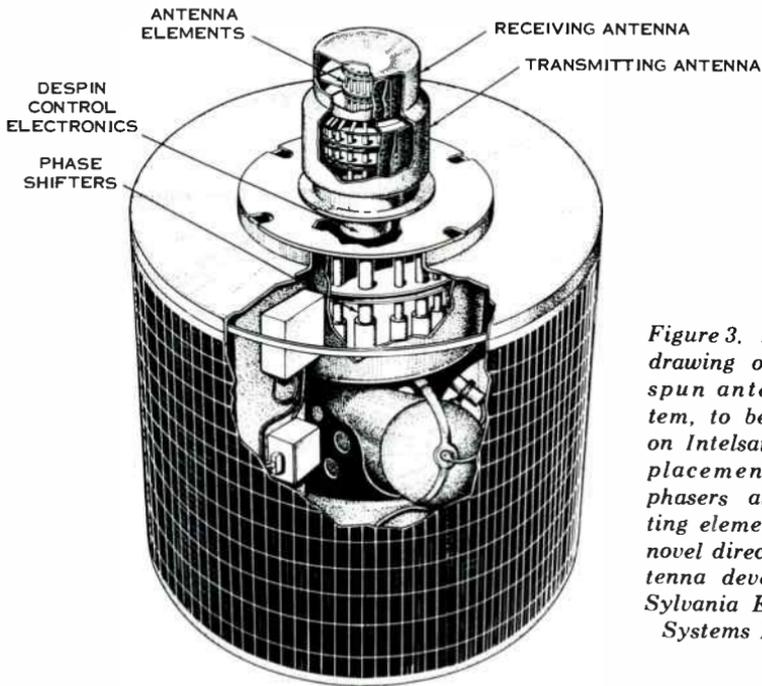
*Figure 3. A cutaway drawing of the despun antenna system, to be initiated on Intelsat 3, shows placement of the phasers and radiating elements of the novel directional antenna developed by Sylvania Electronics Systems Division.*
