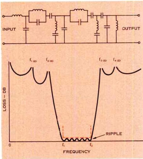
Figure 6. Filter circuit (top) will produce this type of loss-frequency curve. Engineer and computer determine optimum component values to provide proper passband frequencies, acceptable ripple, and infinite loss points.
