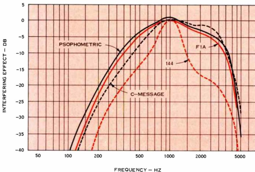
Figure 2. Weighting curves, based on listener response, show the relative interfering effect of noise on speech. All curves are referred to 1000 Hz except psophometric, which is based on measurements at 800 Hz.
