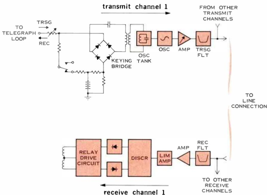
Figure 3. Simplified schematic diagram of telegraph multiplex terminal operating into a half-duplex neutral loop.
