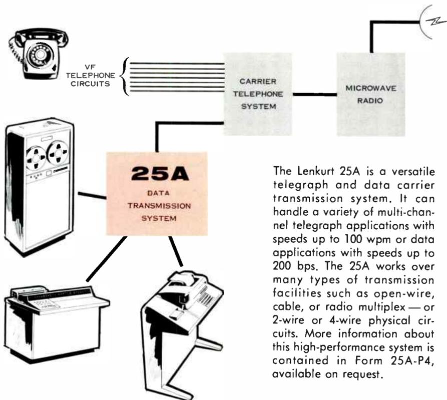
The Lenkurt 25A is a versatile telegraph and data carrier transmission system. It can handle a variety of multi-channel telegraph applications with speeds up to 100 wpm or data applications with speeds up to 200 bps. The 25A works over many types of transmission facilities such as open-wire, cable, or radio multiplex — or 2-wire or 4-wire physical circuits. More information about this high-performance system is contained in Form 25A-P4, available on request.
