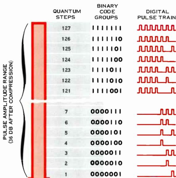
Figure 3. In PCM, amplitude samples of speech signals are compressed, quantized, coded into binary form, and placed on the line as digital pulses.
