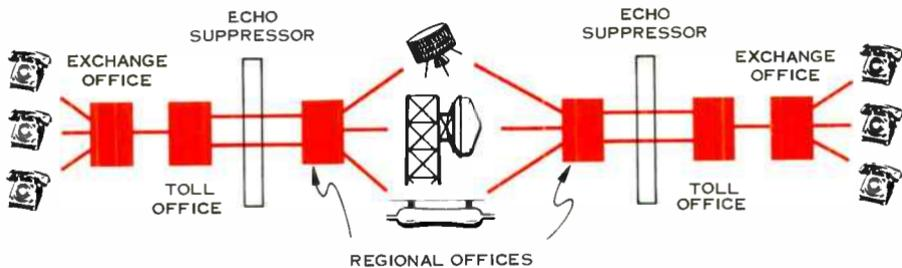
Figure 1. Telephone path through exchange, toll and regional offices. Echo suppressor is located at the beginning of 4-wire toll circuits.
