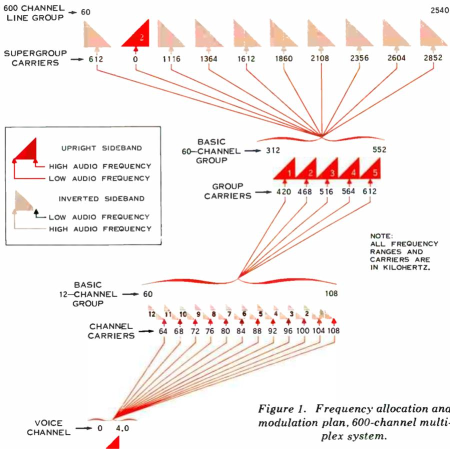
Figure 1. Frequency allocation and modulation plan, 600-channel multi-plex system.
