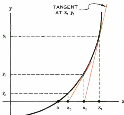
Figure 5. Computer uses iteration to find the point where curve crosses  $x$  axis.
