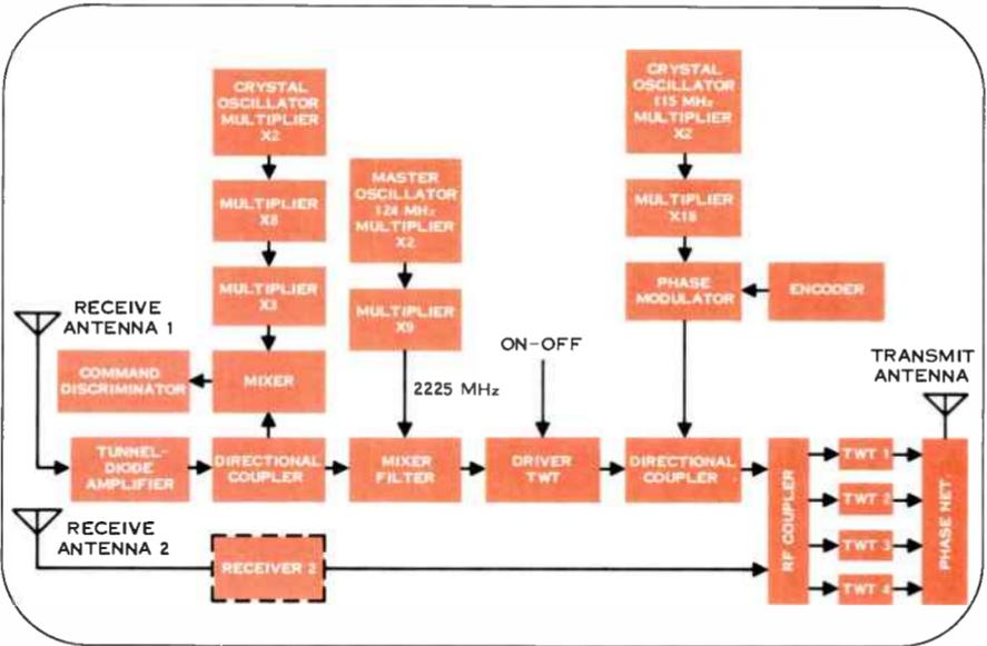
Figure 5. Communications system block diagram for Intelsat 2, built by Hughes Aircraft Co.
