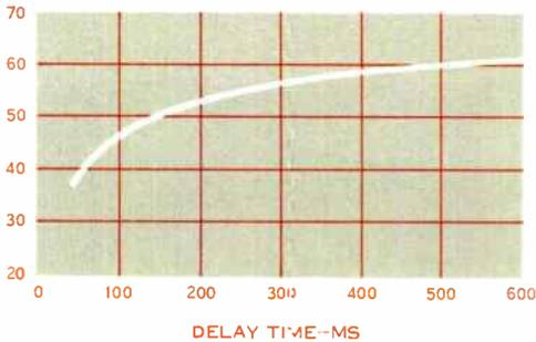
*Figure 3. The attenuation needed to suppress echoes to tolerable levels is indicated for the average telephone talker.*
