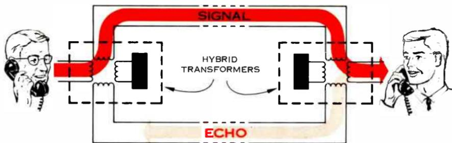
Figure 2. Hybrid transformers are needed at each end of a 4-wire circuit. Reflected energy at this point becomes echo.
