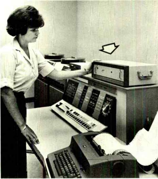
*Figure 4. Data communications terminal (arrow) permits fast and reliable transmission at 2400 bits per second from a central computer.*
