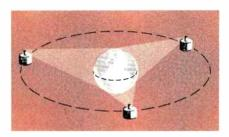
Figure 1. Three satellites in synchronous orbit could cover the entire earth.
