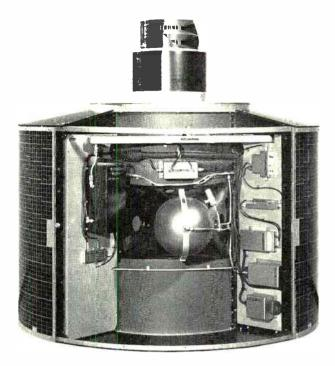
Figure 6. Seen inside Intelsat 3, to be launched in 1968, are many of the electronic and propulsion systems included in the third generation communications satellite being built by TRW Systems.
