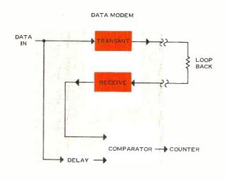
Figure 2. Typical method for measuring error performance of a data communications set. Data signals are looped back from transmitter to receiver. Delay corres. ponding to the amount in the path is added to the original data signals which are then compared bit-by-bit with the received data signals. An error counter keeps track of the number of errors.
