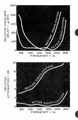
Figure 1. Both delay and amplitude distortion affect the quality of data transmission. Top panel shows the relative envelope delay of a typical voice channel both before and after equalization. The result of amplitude equalization is shown in bottom panel.
