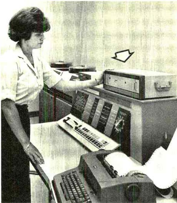
*Figure 4. Data communications terminal (arrow) permits fast and reliable transmission at 2400 bits per second from a central computer.*
