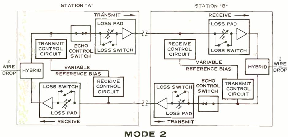
Figure 4. Simplified diagram of Mode 1 (uni-directional) and Mode 2 (bi-directional) operation of the Lenkurt 931B Echo Suppressor.
