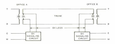
Figure 2. There are a number of different circuit arrangements designed for E & M signaling over telephone tranks. The three most prominent d-c arrangements are: (A) simplex. (B) composite, and (C) duplex.
