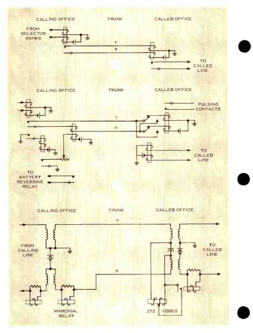
Figure 1. Loop signaling is accomplished by altering the flow of current in the trunk conductors. Three methods used to accomplish loop signaling are: (A) wet-dry, (B) reverse battery, and (C) high-low.
