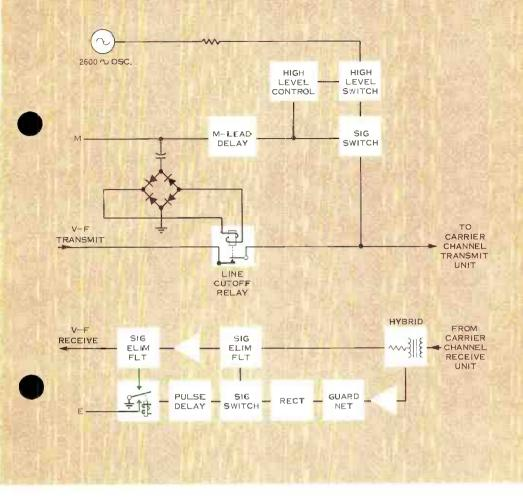
Figure 3. Simplified block diagram of a 2600-hz in-band signaling circuit applied to transmit channel and receive channel of a carrier system.
