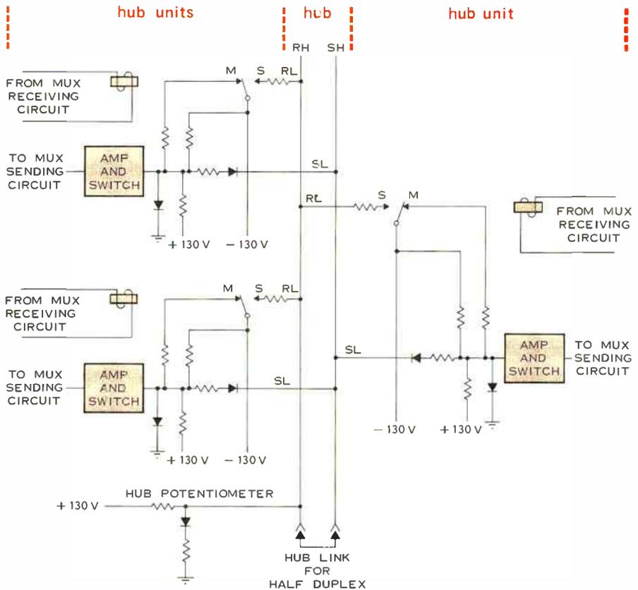
Figure 5. Hub operation, showing three multiplex telegraph channels interconnected on the d-c loop side.
