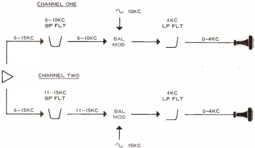
Figure 3. Simplified two-channel telephone multiplex system.
