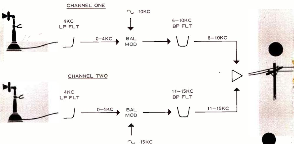
rection of transmission. This permitted the use of filters to separate the channels and the hybrid coils were no longer necessary. This technique of using different frequencies for each direction provided what is known as an *equivalent 4-wire* system.
