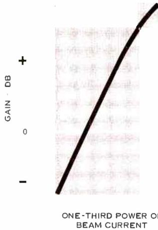
Figure 7. Gain vs. beam current.
