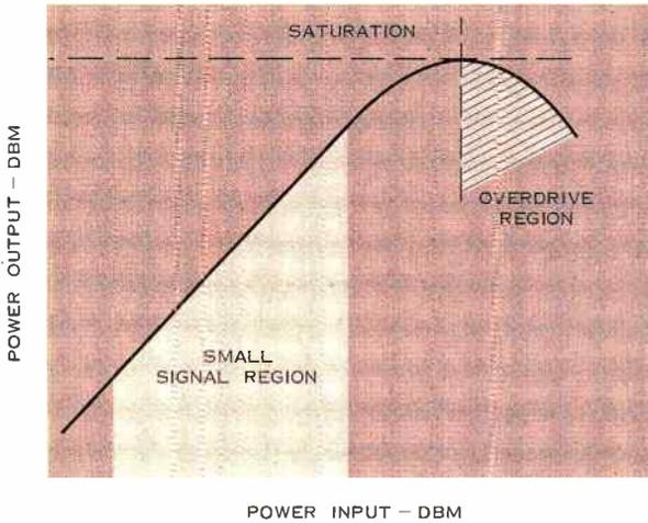
Figure 5. Power output vs. power input.
