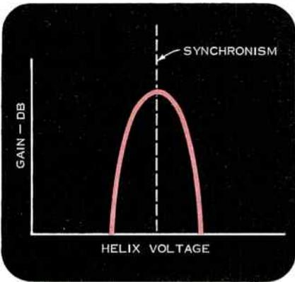
Figure 6. Gain vs. helix voltage.
