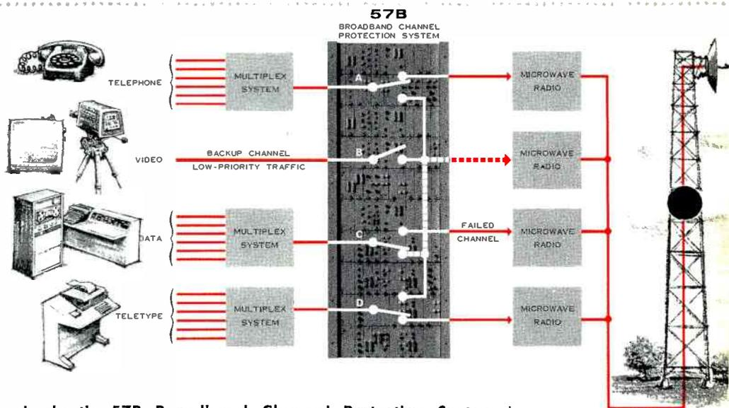
Lenkurt's 57B Broadband Channel Protection System is an economical and efficient method of improving the path reliability of microwave radio links. One radio channel can be used to provide stand-by protection for up to three other broadband radio channels, carrying higher priority traffic. More information about this economical system is contained in Form 57B-P4, available on request from the Sales Promotion Manager.
