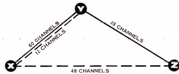
Figure 2. Possible routing for 12 channels between stations X and Y and 48 channels between stations X and Z.
