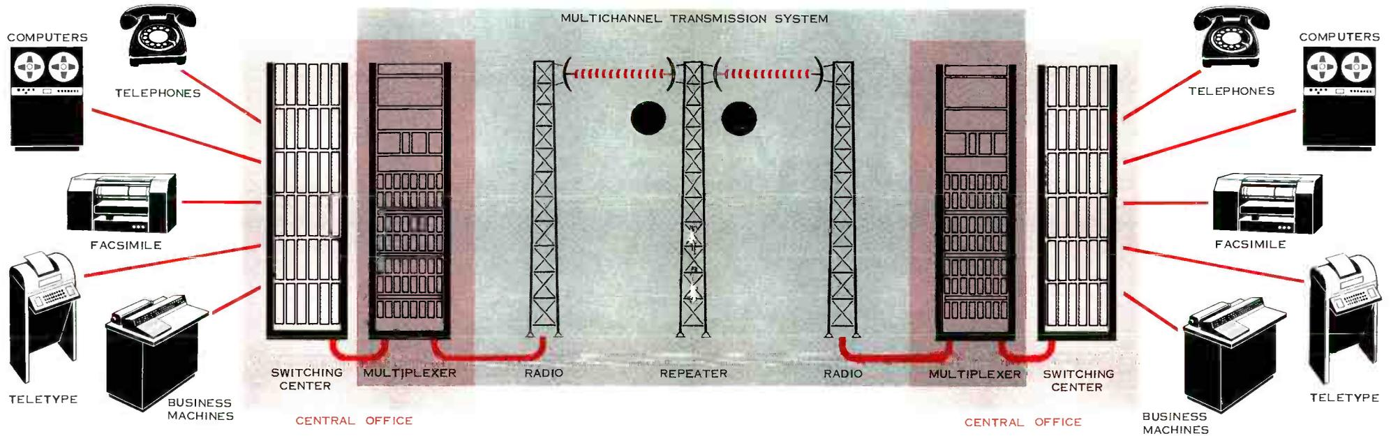
Figure 3. Typical communications network with a multichannel transmission system containing multiplex equipment, microwave radio terminals, and intermediate repeater station.
