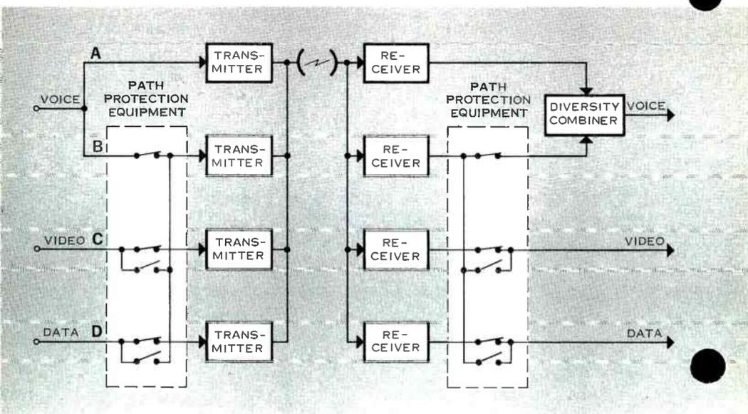
Figure 4. Functional diagram of typical one-for-three broadband radio path protection system.
