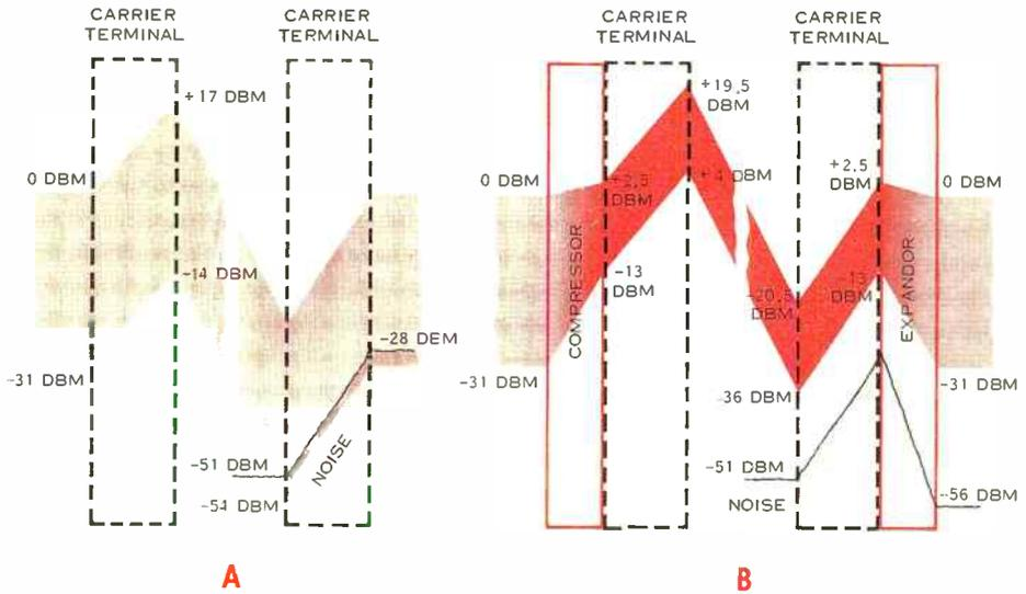
*Figure 6. Using compandors, toll quality transmission can often be achieved over a circuit otherwise unsuitable because of noise. Diagram A shows a typical circuit, without a compandor, where the weakest speech signal at the receiving end is 3 db below the noise level. Diagram B shows the same circuit with a compandor added. The weakest speech signal at the receiving end is now 25 db above the noise level, resulting in a 28 db noise improvement.*
