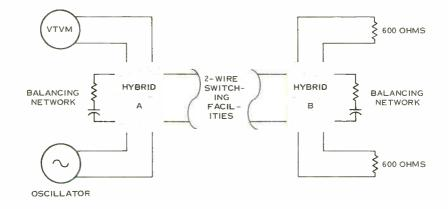
Figure 4. Typical test arrangement for measuring echo return loss. ERL measurement here depends primarily on the quality of the termination which Hybrid B provides for the two-wire line.
