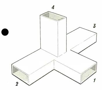
Figure 8. "Hybrid tee," used for microwave frequencies. provides isolation between opposite arms, but maintains low-loss path between adjacent arms. A signal in arm 4 produces equal and opposite signals in arms 2 and 3, nothing in arm 1. With input to arm 1, equal inphase signals exist in arms 2 and 3, with no coupling to arm 4.
