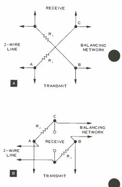
Figure 7. Resistance hybrid as usually drawn (A), and redrawn to illustrate bridge configuration (B). Although less expensive than transformer type, resistance hybrids introduce more transmission loss.
