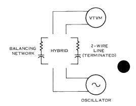
Figure 3. Typical test arrangement for measuring how much isolation the hybrid provides between the branches of a four-wire line. Ideally, no oscillator power would reach VTVM.
