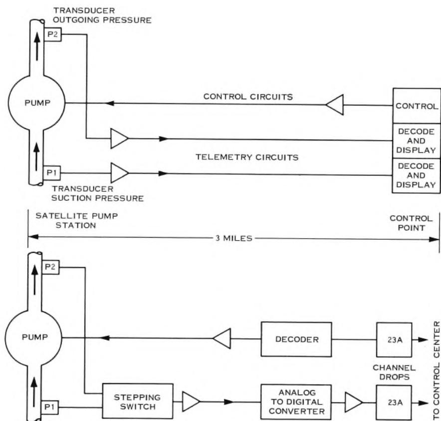
*Figure 4. Oil and gas producing units and pipelines have long used relatively short-range direct-current telemetry to monitor and control satellite operations. Direct current transmission impairs accuracy of telemetry beyond a few miles. Judicious use of analog-to digital converters and modern telegraph carrier permits centralized control over far greater distances without obsoleting existing short-range equipment.*
