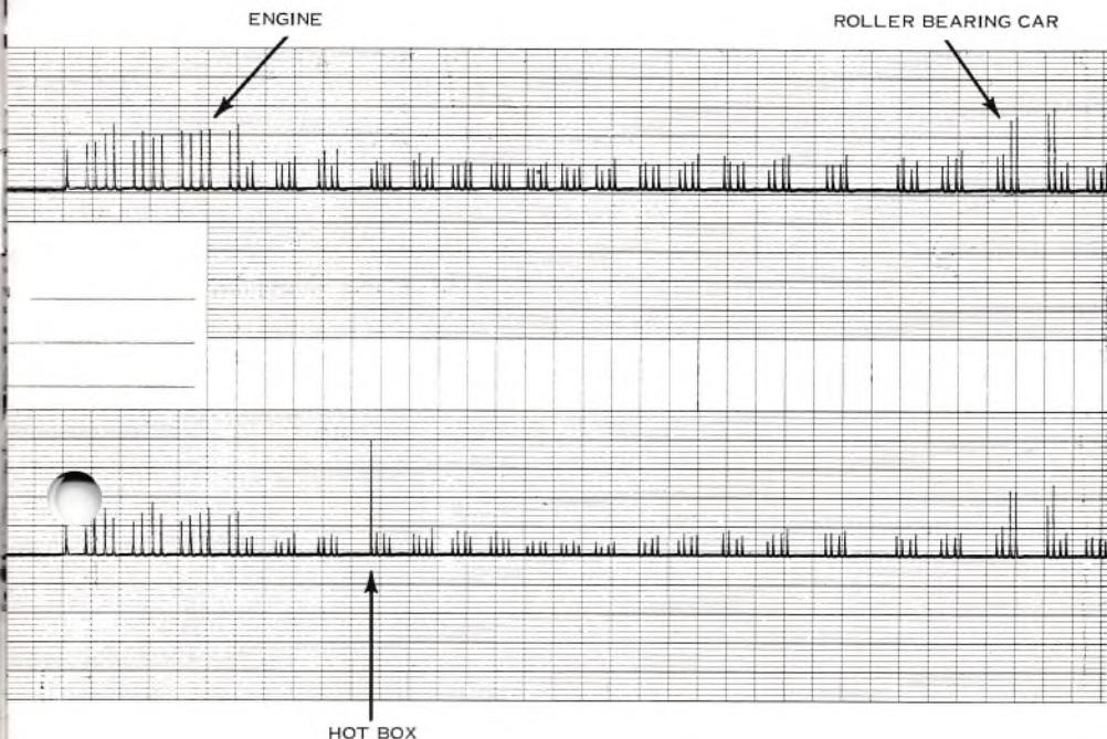
Figure 2. Typical hot-box detector transmission. Each pip shown represents a single wheel. Two recordings are made simultaneously, one for each side. Engine driver wheels, shown at left, and roller bearings always operate at higher temperatures than ordinary solid or plug-bearing journals. Note hot-box indication.
