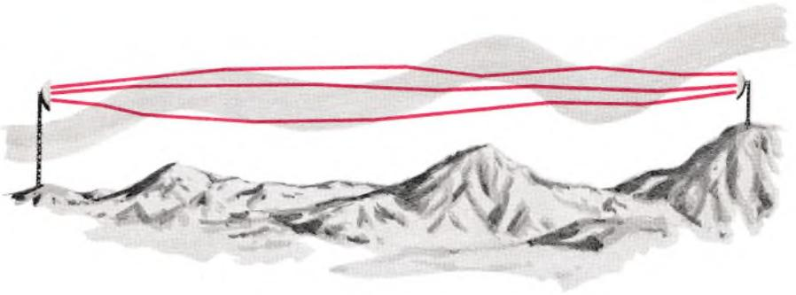
*Figure 3. Irregularities in atmosphere cause radio beam to break up into several components traveling different paths. Those which manage to reach receiving antenna will have traveled paths of different lengths, causing phase cancellation.*
