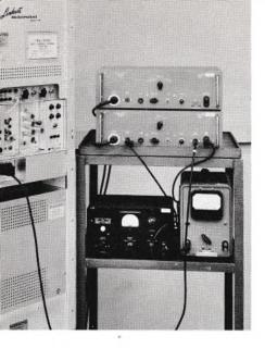
Figure 4. Lenkurt Type 5203-5204 Distortion Test Set in use. This equipment works on principle diagrammed in Figure 3.
