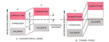
Figure 12. Very heavy doping of n and p semiconductors shift their respective energy levels. Applied forward bias tends to reduce difference between two. When valence band of p material is directly opposite conduction level of n material, current carriers may "tunnel" through potential barrier at speed of light. Increased forward bias shifts n valence band opposite p forbidden zone, restoring normal diode behavior.
