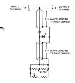
Figure 5. Tunnel diode equivalent of circuit shown in Figure 3. This amplifier is designed for UHF service, requires transmission-line transformers for impedance match between 50-ohm line and much lower impedance tunnel diode.
