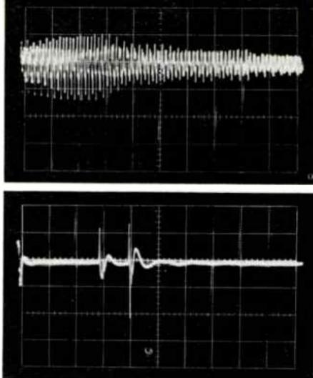
Figure 2. Comparison of speech and noise impulse recorded from actual telephone circuit. Speech sample is the word "two." Note slight ringing following each noise impulse.
