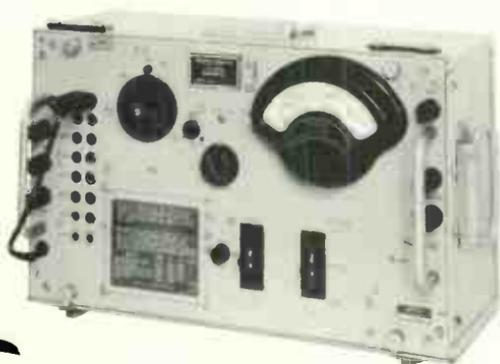
Figure 3. A typical noise measuring set used for determining noise characteristics of communications channels. Instrument permits noise measurements under wide range of conditions and with any of several line weightings.
