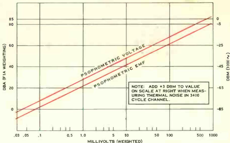
Figure 6. Comparison of dba and psophometric noise values. Dba is logarithmic unit, while psophometric noise values are linear.
