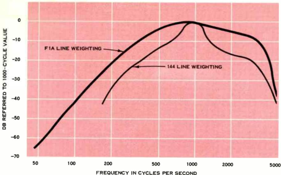
Figure 4. Weighting curves show the relative interfering effect of noise on speech when using either Type 144 or F1A handsets or their equivalents. F1A curve is international standard.
