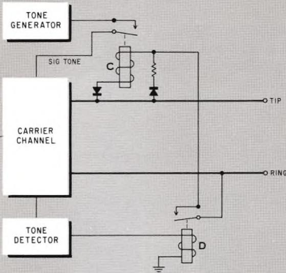
*Figure 3. Typical arrangement for single-tone signaling over carrier channel between exchanges.*
