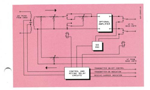
Fig. 2. Simplified schematic diagram of a manual mobile telephone control terminal.
