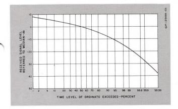
Fig. 1. The Rayleigh distribution shown is used to predict radio signal level variations which may be expected to occur over a well-engineered radio path.
