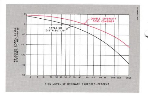
Fig. 3. Radio signal level distribution of the Type 5055 Combining and Transfer Panel is compared to the Rayleigh distribution. The signal level difference between the two curves is the Diversity Advantage.
