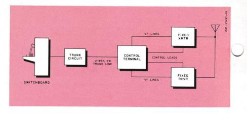
Fig. 1. Block diagram of the base station equipment showing interconnection to central-office switchboard.
