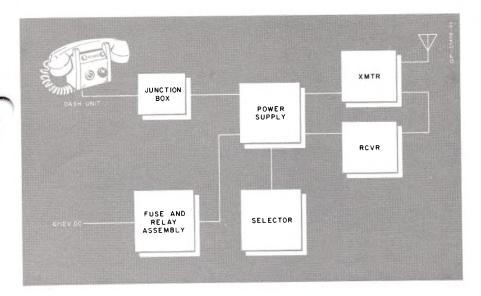
Fig. 4. Block diagram of a typical mobile subscriber station.
