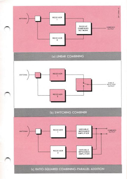
Fig. 2. The three basic combining methods shown in block schematic form.
