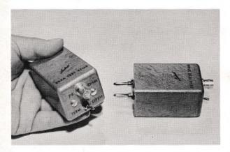
Illustrated above is the Type 583A Test Transformer. The transformer in the 583A is designed for impedance matching between 600- and 75-ohm circuits, and facilitates measurements made in radio circuits with 600-ohm test equipment. Banana plugs are provided at one end for connection to test oscillators or vacuum-tube voltmeters. A coaxial connector at the other end permits patching to coaxial circuits with a test cord such as the Lenkurt Type 693A.
