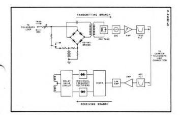
Fig. 2. A simplified block and schematic diagram of a 23A telegraph and data FS carrier channel operating into a half-duplex neutral loop. Frequency shift is controlled by voltage combinations obtained from local battery and the loop. Fig. 3. Eighteen telegraph channels are applied to one carrier telephone channel. Other carrier channels may be used for message circuits or telegraph or data carrier channels.
