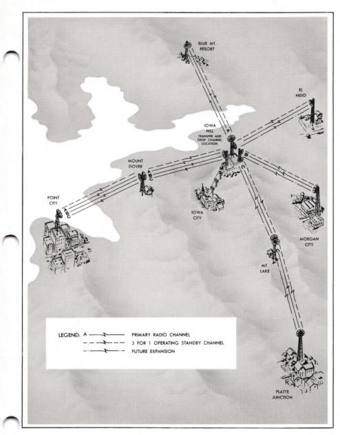
FIG. 7. A possible network of Type 74A microwave equipment using one standby channel for three operating channels.
