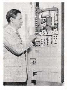
FIG. 1. A basic terminal of Microtel equipment consisting of a transmitter, receiver, and power supplies.
