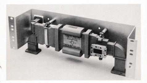
FIG. 3. The waveguide ferrite circulator designed specifically for the Type 74A Radio System. This device permits three microwave terminals to be connected to the same antenna without mutual interference.
