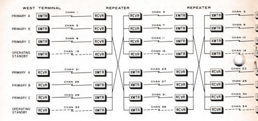
FIG. 6. Frequency assignment plan for a plan, each radio-frequency chann
