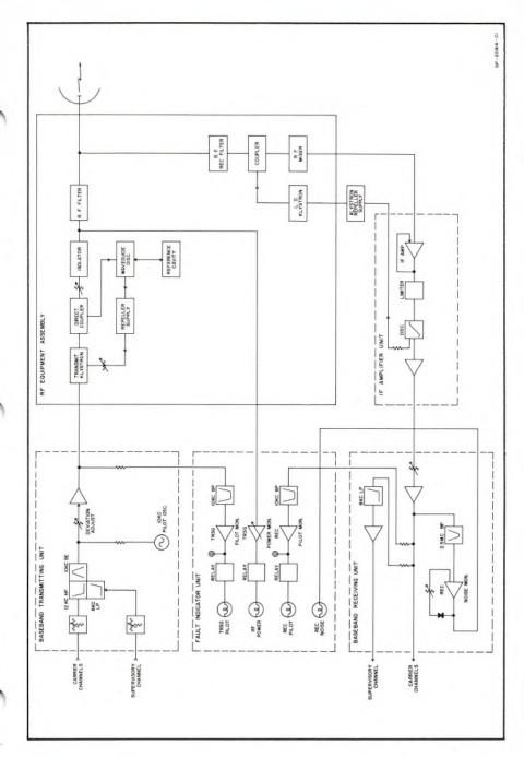
FIG. 5. Simplified block diagram of a Microtel terminal. When standby equipment is furnished, a terminal also includes a combining and transfer unit and a ferrite circulator.
