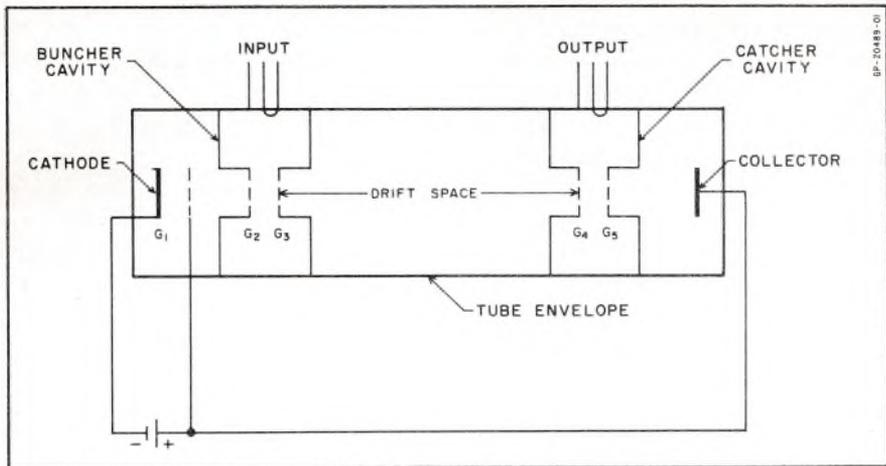
FIG. 1. Simplified diagram of a klystron amplifier. An actual klystron usually has a set of electrodes at the cathode which focuses into a narrow beam.
