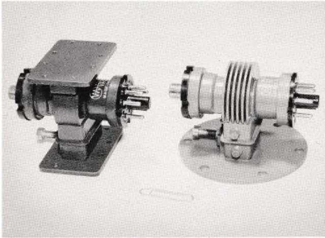
*FIG. 3. Two typical reflex klystrons. The one at left is rated at one watt, and the one at right, at 35 milliwatts.*
