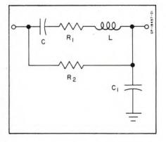
FIG. 3. The equivalent circuit of a capacitor.
