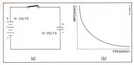
FIG. 2. (a) A circuit in which electric charge has built up in a capacitor opposing the flow of current from the d-c source. When steady state has been reached, no current can flow. (b) The impedance-frequency characteristic of a capacitor.
