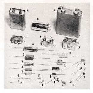
FIG. 1. Types of capacitors used in Lenkurt carrier and microwave radio equipment. Letters indicate dielectric as follows:
