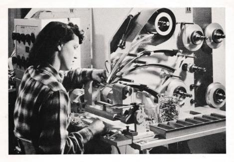
FIG. 4. Automatic machine used for winding polystyrene capacitors at Lenkurt.
